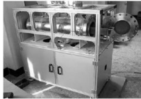
Fig. 2. Pressure treating cylinder.
