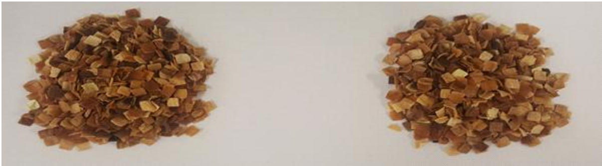
Fig. 3-32. Effects of water vaporization-combined CP treatment on the appearance of onion powder. Representative images of untreated onion powder (left) and treated onion powder (right) are shown. The plasma-forming gas, treatment voltage, frequency, and time were helium, 9 kV, 15 kHz, and 20 min, respectively.
