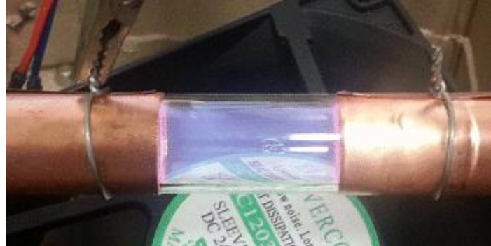
Fig. 3-19. Quarts-copper electrodes used in a preliminary study
