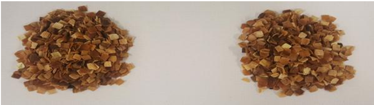
Fig. 21. Effects of water vaporization-combined CP treatment on the appearance of onion powder. Representative images of untreated onion powder (left) and treated onion powder (right) are shown. The plasma-forming gas, treatment voltage, frequency, and time were helium, 9 kV, 15 kHz, and 20 min, respectively.
