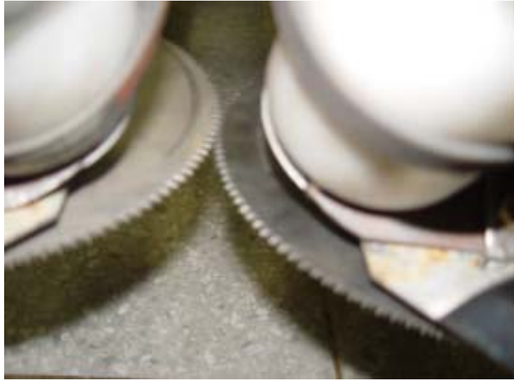
Figure 16. Photograph of circular saws of reaping unit of garlic bulbils collecting system.
