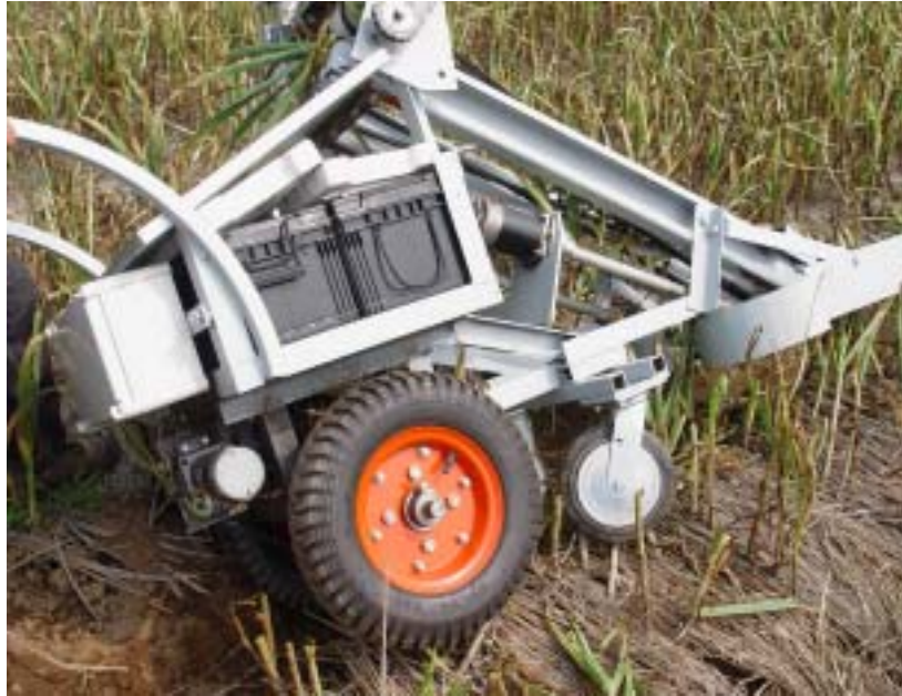
Figure 33. Photograph of overturned prototype garlic bulbils collecting system before modified.
