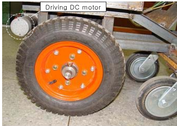
Figure 22. Photograph of the first designed traveling unit of the prototype garlic bulbils collecting system.
