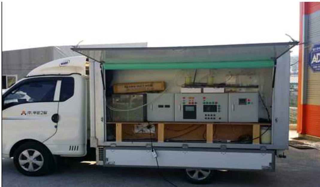
Fig. 13. The large-scale chlorine dioxide gas generating machine
