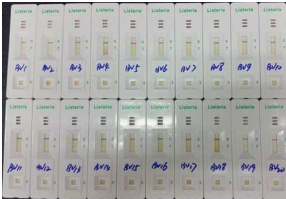
Figure 8.20 Validation results for lettuce inoculated with L. monocytogenes ATCC 19114 A) MOX agar results for low level and high level inoculum (each 10 samples); B) rapigen kit results for low level and high level inoculum (each 10 samples)
