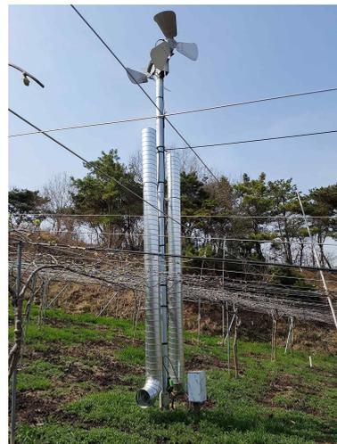
Fig. 14. Fan built in kiwifruit orchard to prevent frost injury.
