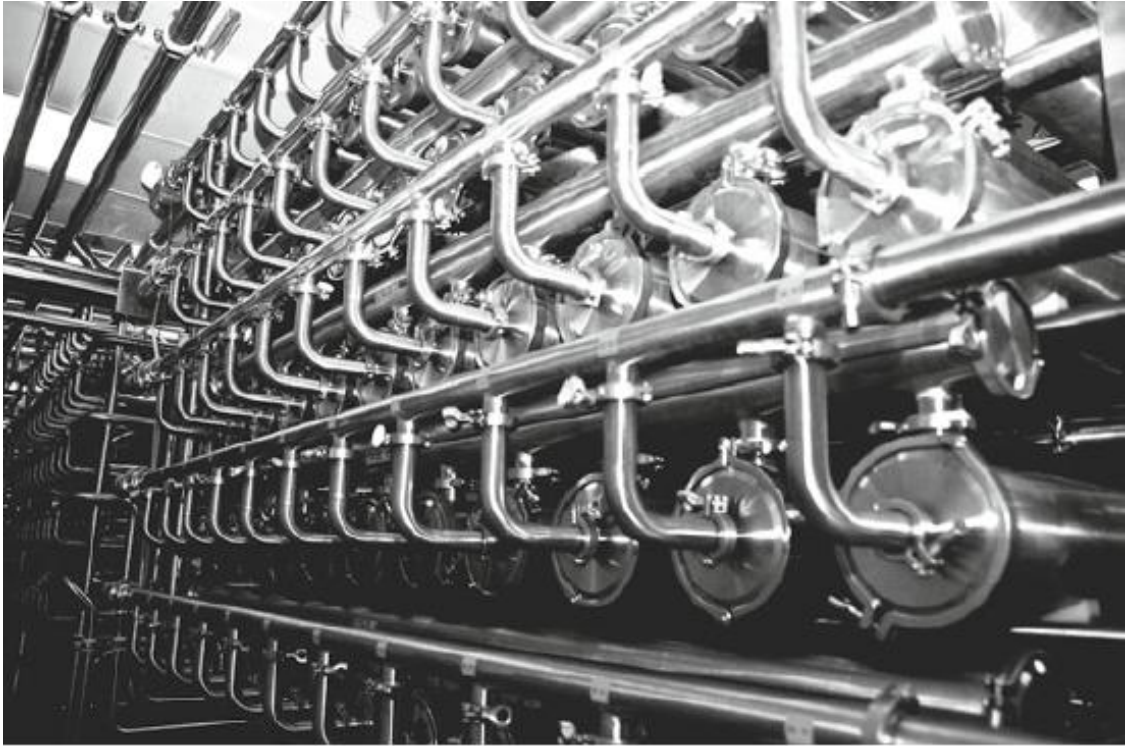
Fig. 3-1-4. Ultra filtration system (Courtesy: Milk Specifications Global)
