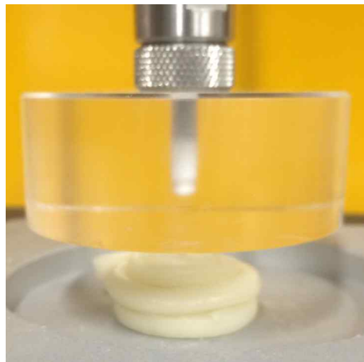
Fig. 3-3-40. Method of texture analysis of noodle.
