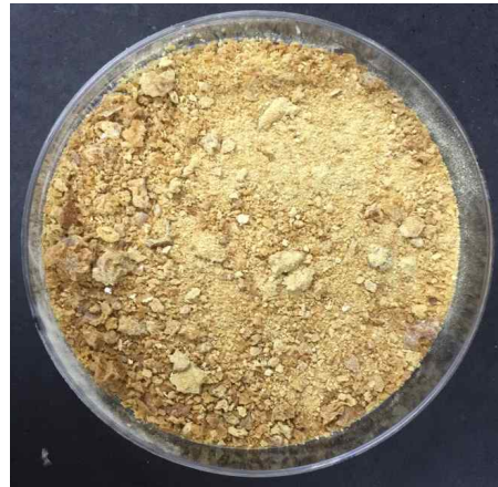
Fig. 3-3-51. HAP powder above 5 kDa manufactured by freeze dryer.
