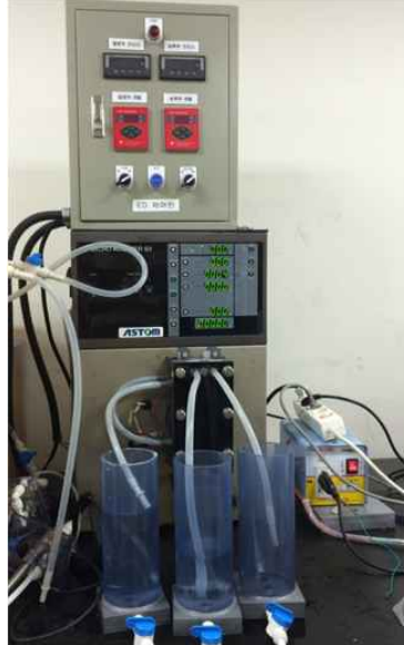
Fig. 3-1-41. 전기투석 장비(Micro-acilyzer S3, Astom, Japan).
