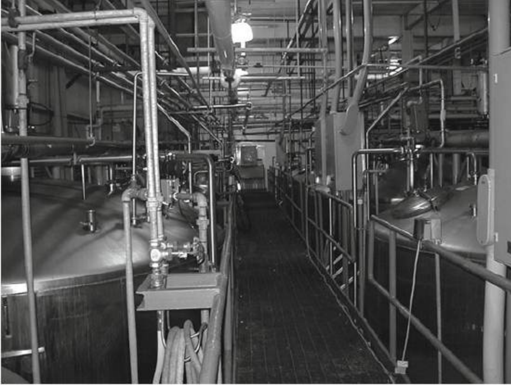
Fig. 3-1-3. Bank of hydrolysis reactors (Courtesy: Kerry Biosciences).
