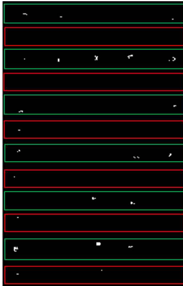
그림 86. Online sorting results of white corn based on PLS-DA with conveyor speed 30rpm (4.16cm/s).
