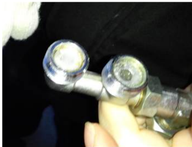
Figure 68 Ice in the nozzle
