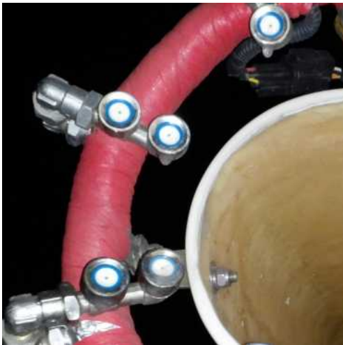
Figure 67. Icicle forms at nozzle
