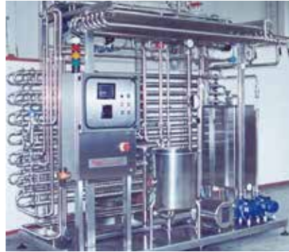
【그림 6-6】 Flash pasteurisation 살균기(KHS machine manufacturing and engineering, Dortmund)
