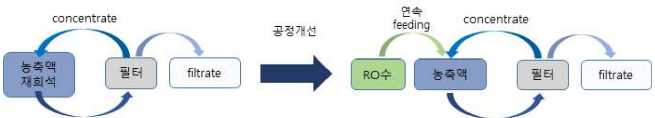
Fig. 3-41. Schematic diagram of continuous UF process
