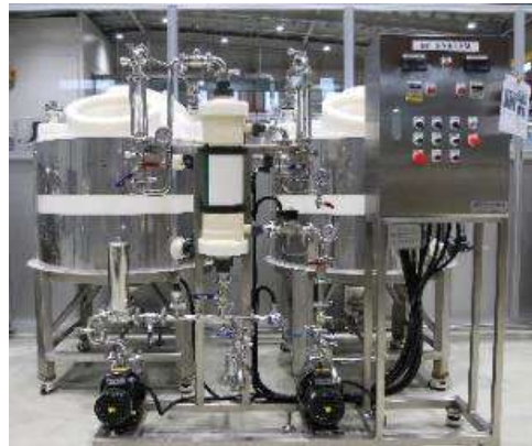
Fig. 4-33. MF/UF system for pilot-scale production of \beta -limit dextrin
