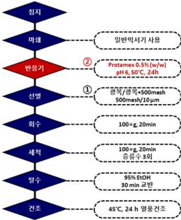
Fig. 1-18. Schematic diagram from rice starch production using protease.
