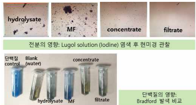
Fig. 3-44. Analysis of the fouling in microfilter adapted in UF system
