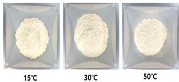
Fig. 1-19. Appearance of rice starch isolated under different temperature of protease treatment from milled rice.
