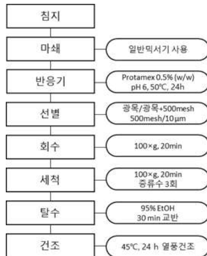
Fig. 1-14. Schematic diagram for preparing rice starch by enzymatic method.
