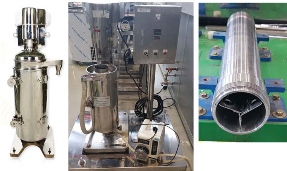
Fig. 3-16. Continuous centrifugation model used for isolation of rice starch
