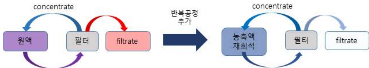
Fig. 3-39. Schematic diagram of repetitive UF process
