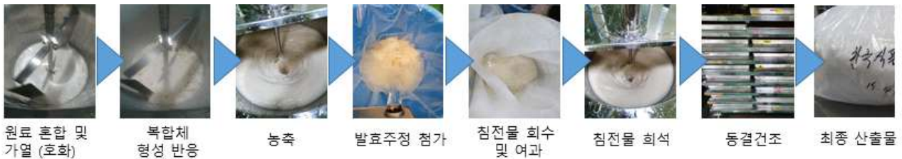
Fig. 3-50. Mass-production of complex between \beta -limit dextrin and lipid
