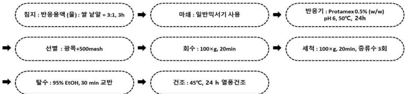
Fig. 1-20. Optimal production process of rice starch from broken rice using protease.
