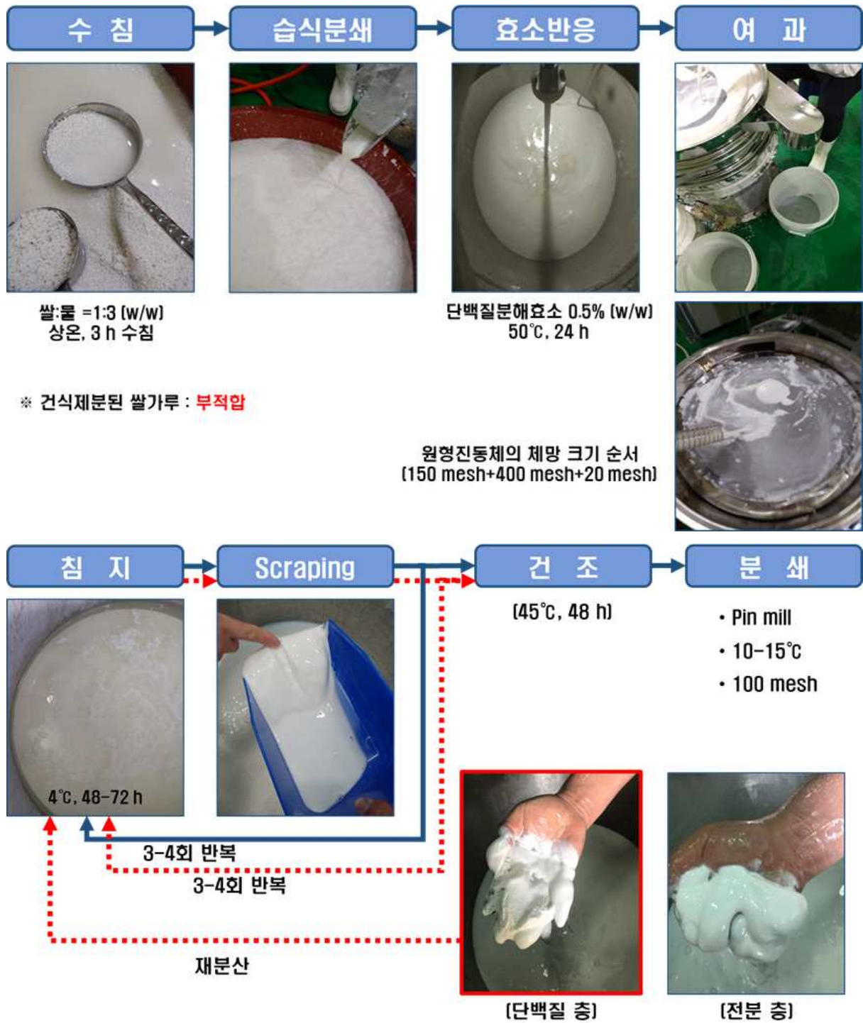
Fig. 1-35. Mass production process of rice starch using the improved enzymatic method.
