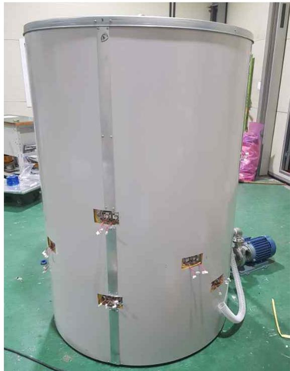
Photo after installing ceramic heater (4)
