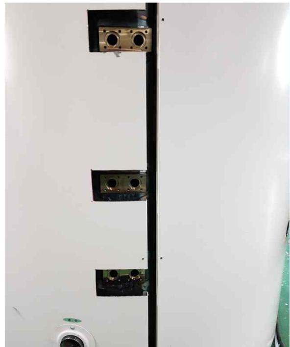
Figure 74. Installation of ceramic heater fixing jig in water tank
