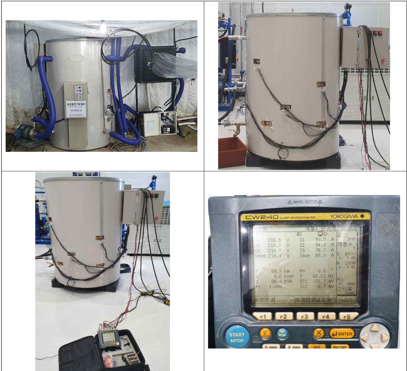
Figure 118. Measurement of power consumption of agricultural electric boilers (Measurement Institution: Agricultural Technology Commercialization Foundation)
