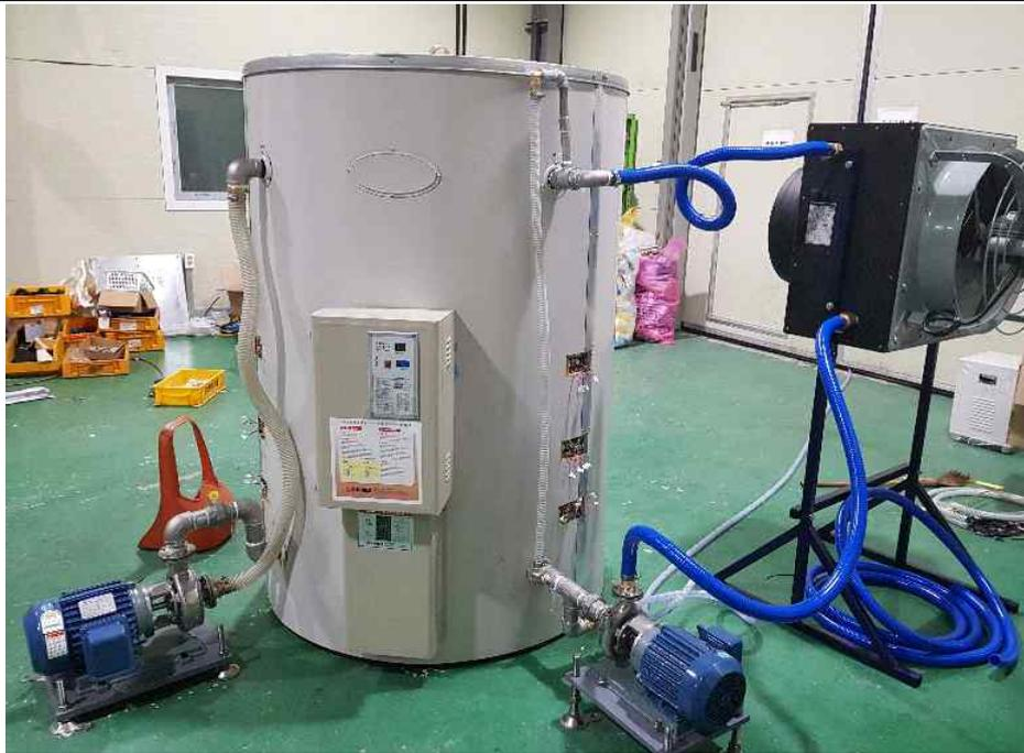
Figure 121. Installation of a pump for circulation of an internal flow path of an agricultural electric boiler
