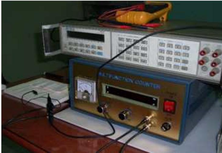
Figure 56. Ceramic Heater Power Consumption Measurement System
