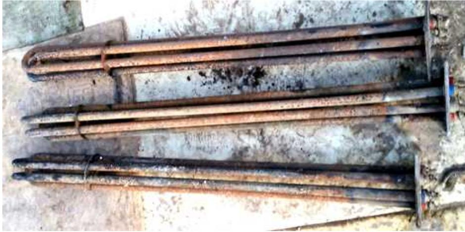
Figure 114. Sheath heater for conventional agricultural electric boilers
