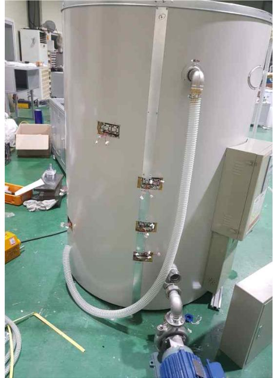
Photo after installing ceramic heater (2)
