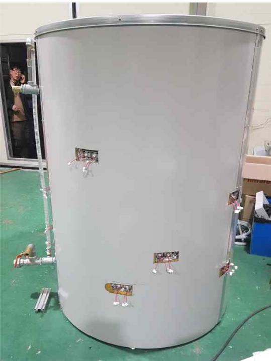
Photo after installing ceramic heater (3)
