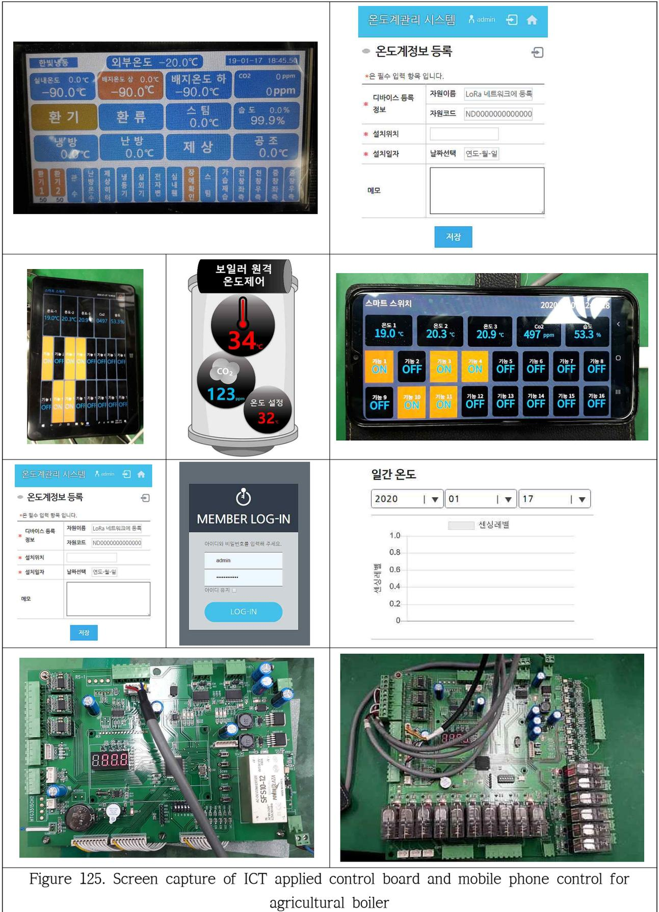
Figure 125. Screen capture of ICT applied control board and mobile phone control for agricultural boiler
