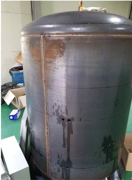
Figure 71. Picture of water tank welding and drilling of heater part
