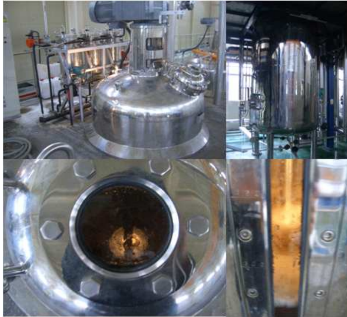
Fig. 12. 5,000 liter plant scale fermenter used in the study
