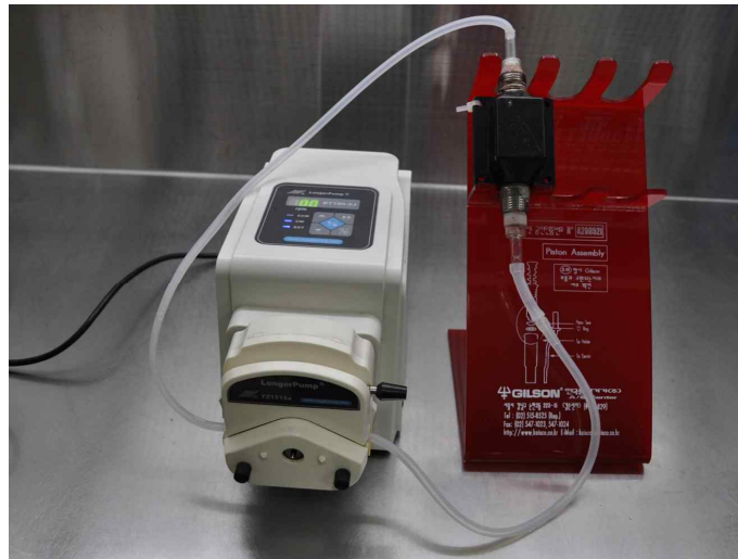
Fig. 2. Image of magnetic equipment system, left equipment is Peristaltic Pump, right equipment is neodymium magnet
