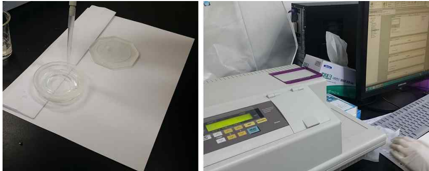
Fig. 44. Analysis of VBN using spectrophotometry
