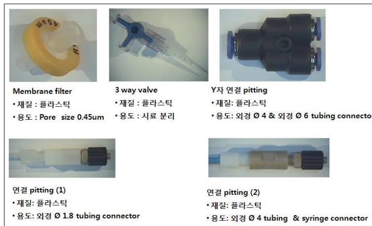
Fig. 71. Membrane filter, 3 way valve and solution outlet parts.
