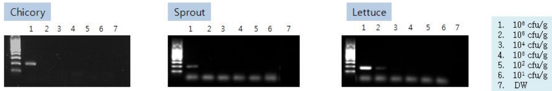
Fig. 67. Electrophoresis of real-time PCR products by lab-on-a chip NBS-100 system in artificially inoculated vegetables.
