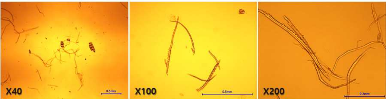
<Fig. 2.68> Microscopic image of rice husk kraft pulps under active alkali of 25%.
