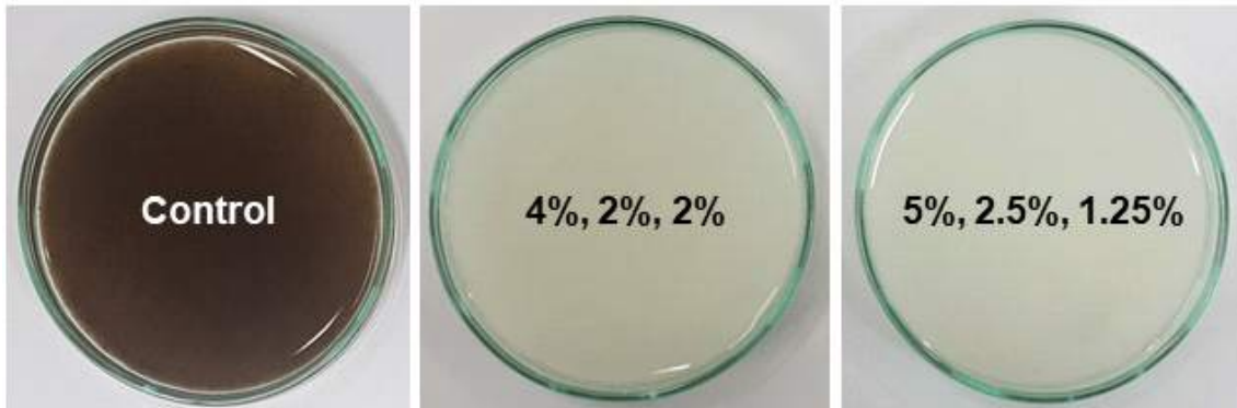
<Fig. 2.85> Persimmon byproduct pulps as a function of D-E-D bleaching chemical addition.
