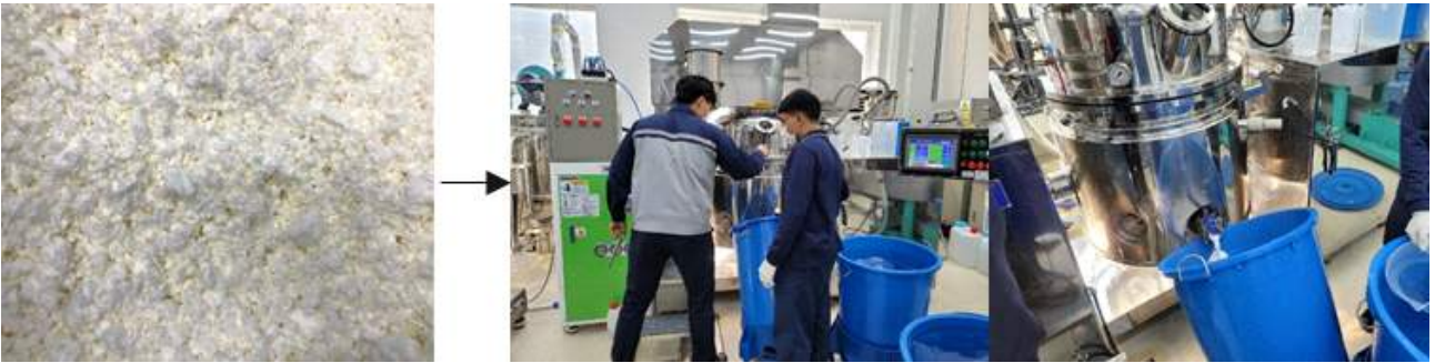
<Fig. 2.369> CNF manufacturing process of Moorim P&P : mixture of bamboo and hardwood BKPs(left) and enzyme pretreatment(right).
