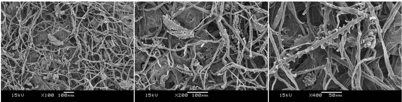
〈Fig. 2.71〉 SEM images of the rice husk kraft pulp at strong pulping condition.
