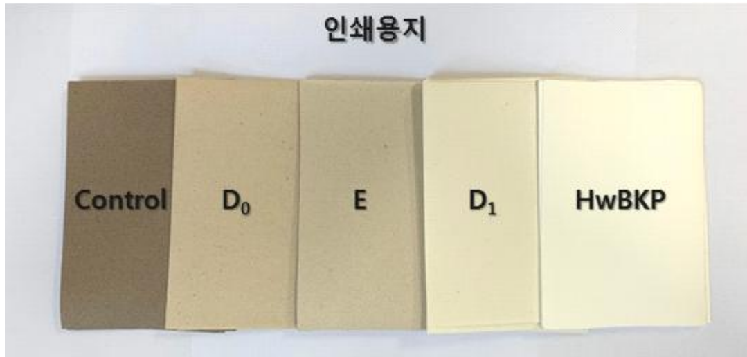
<Fig. 2.155> Appearance and color of handsheet as a function of bleaching steps and pulp type.
