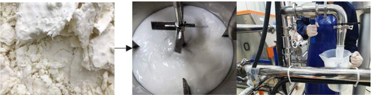
<Fig. 2.370> CNF manufacturing process of Moorim P&P : enzyme pretreated BKP mixture(left) and homogenizing process after enzyme pretreatment(right).
