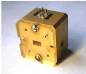
8 mm range voltage-controlled oscillator
