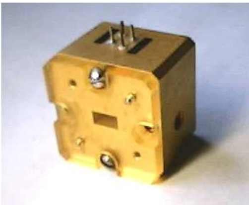
Voltage-controlled oscillator of 8mm range
