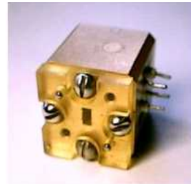
5 mm range voltage-controlled oscillator on Gunn diode
