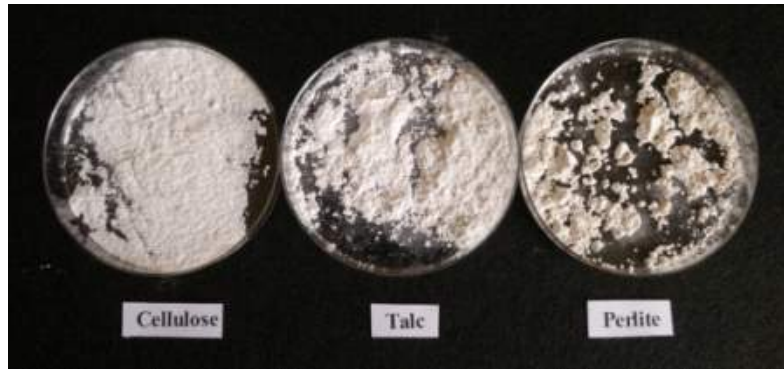
Fig. 2.48. Coating materials: cellulose (Daejung chem. microcrystalline), talc(Nongwoobio), and perlite (green pamix 200 mesh).
