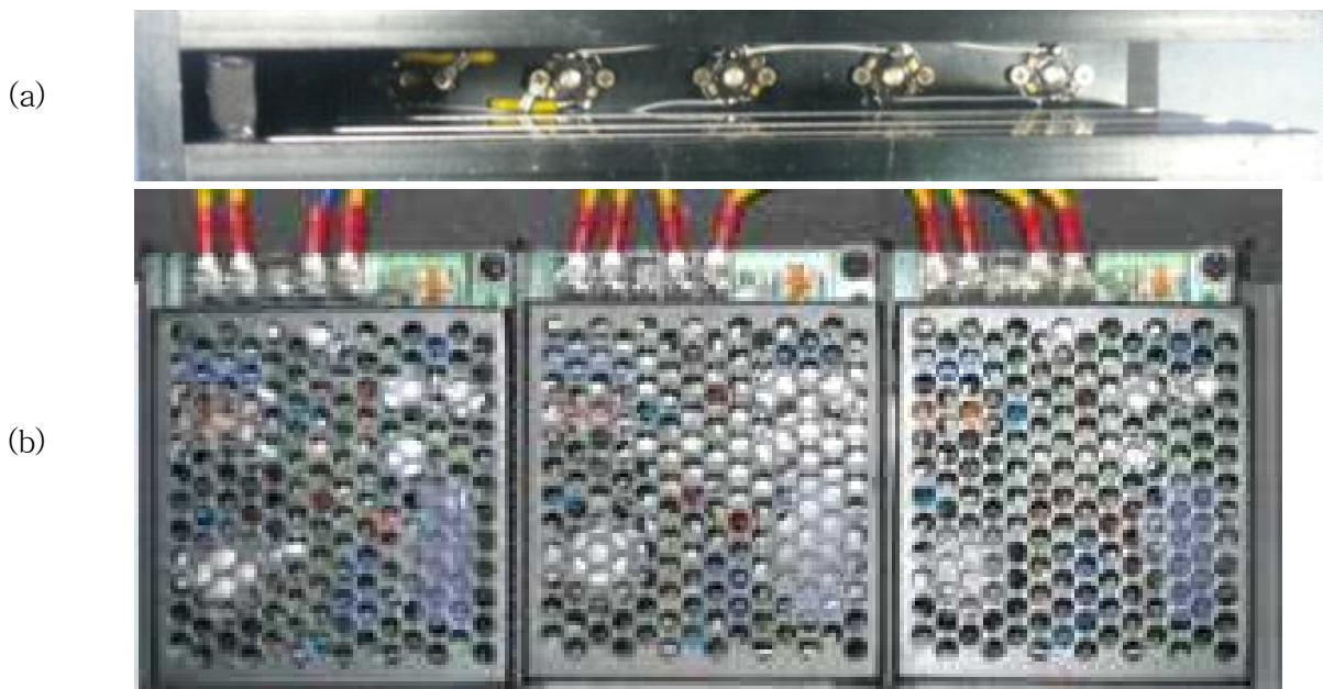
Fig. 4.24. Photo of the installed power LEDs (a) and the switched-mode power supplies of 24 V.
