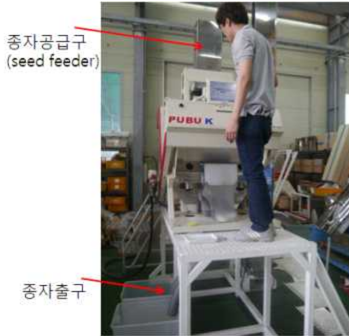
Fig. 2.60. Color sorter (Model: PUBU-K) and working on seed separation.
