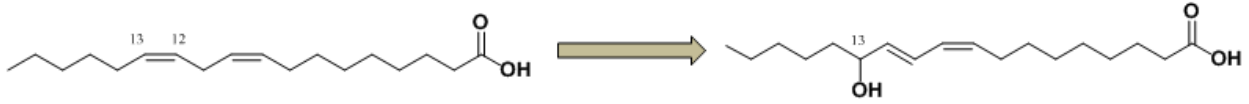
Fig. 16. Scheme of 13-hydroxy-9Z,11E- octadecadienoic acid (13-HODE) production from linoleic acid using 9-lipoxygenase.
