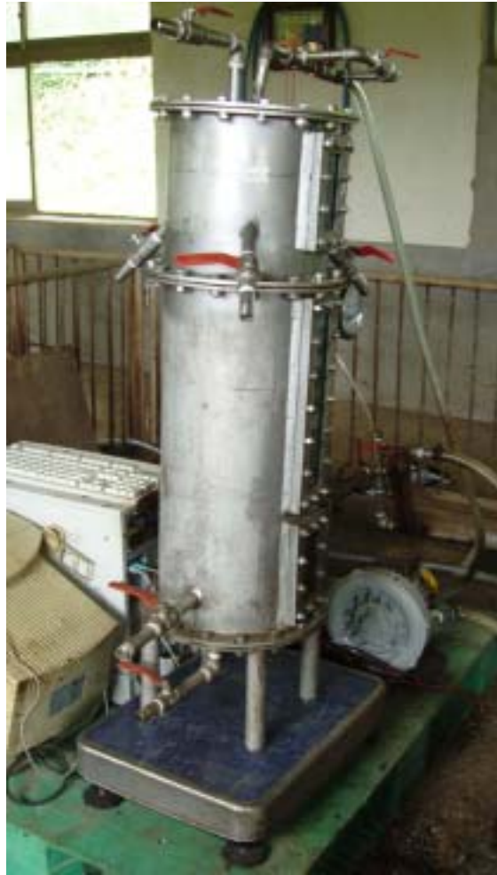
Fig. 3.1.22. Pilot-scale biofilter system <Model C> operating for the pigsty.
