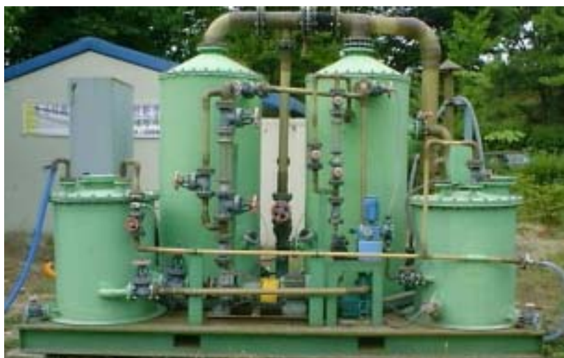
Fig. 3.2.24. Overall appearance of the pilot-scale biofiltration system <Model B>, which provided by KavoTech Co. Ltd. for these experiments.
