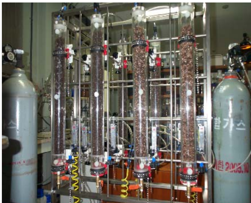
Fig. 3.1.1. Lab-scale biofilter<Model A-1> sets for enrichment of the ammonia and hydrogen sulfide oxidizing microorganisms. Packing materials were: wood bark (composted chaff of pine) 15, perlite 1, compost-I 2, compost-II 1 L; moisture contents during operation 49.2~61.1%. Average concentration of influent NH 3 gas 102.7 ppm v ; flow rate 4,000 mL min -1 , and that of influent H 2 S gas 58.4 ppm v ; flow rate 2,000 mL min -1 .
