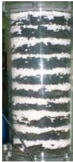
Fig. 3.1.13. Column packed with the mixed material consisted of composted chaffs of pine and perlites.
