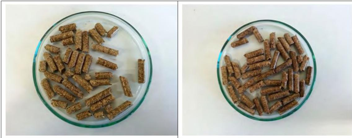
그림 3-3-18. Images of pellets produced with 100% rape stalk (left) and 90% larch sawdust/10% no immersed rape stalk (right).
