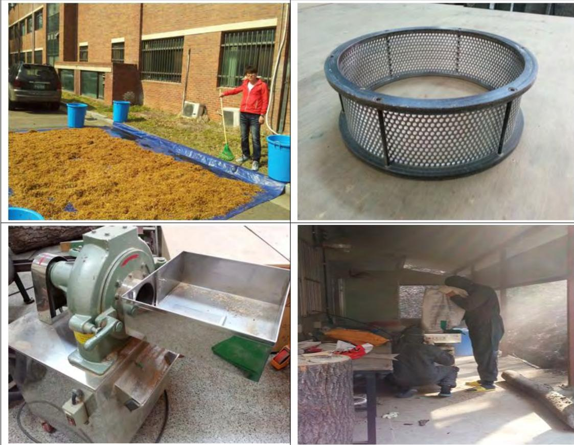
그림 3-3-16. Drying of immersed rape stalk (top-left) and images of milling machine and milling process (bottom-right).
