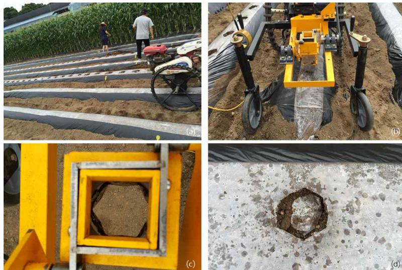
Fig. 144. Field test (crank type), (a) Punching operation, (b) Punching round knife, (c) Changing knife, (d) Hexagonal cutting shape of plastic mulching
