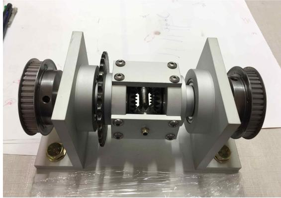
Fig. 212. Automatic transmission of 3<sup>rd</sup> year automatic punching machine prototype, from working machine to punching machine
