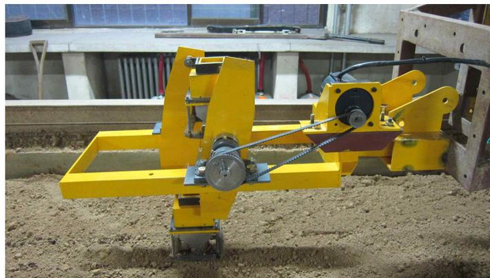
Fig. 114. View of the circular-path type puncher
