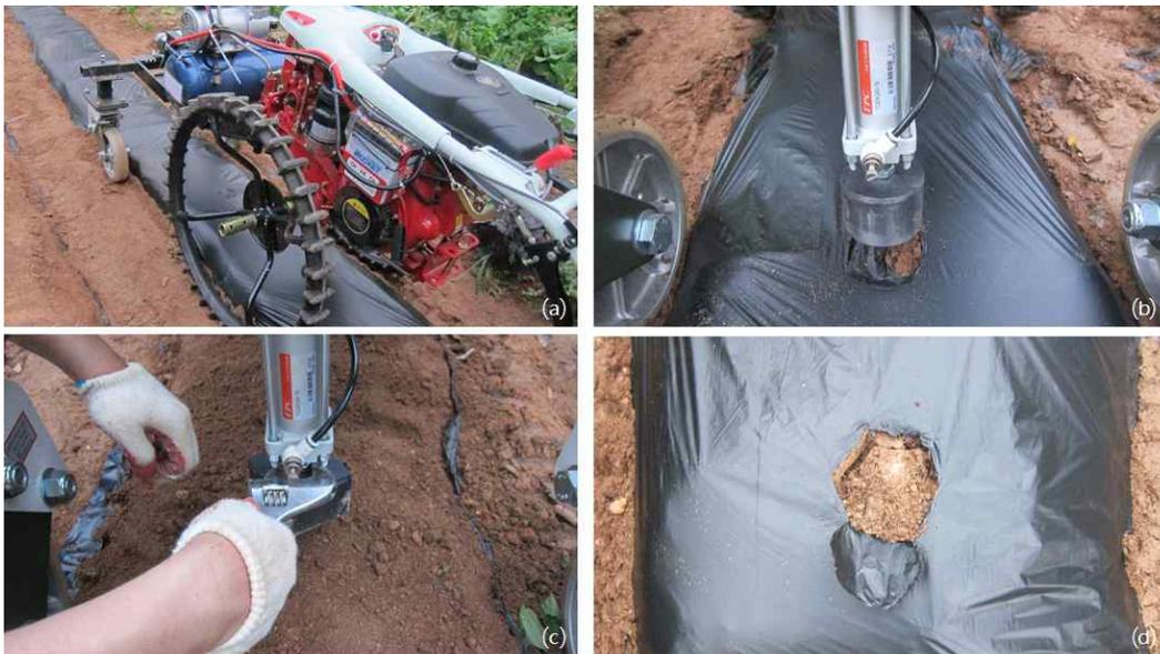
Fig. 152. Field test (cylinder type), (a) Punching operation, (b) Punching round knife, (c) Hanging knife, (d) Hexagonal cutting shape of plastic mulching
