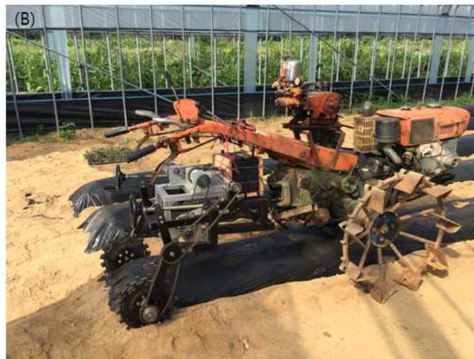
Fig. 215. 3<sup>rd</sup> year automatic punching machine prototype, (A) attached to agricultural working machine (Asia-Tec, AMC-880), (B) attached to agricultural tiller
