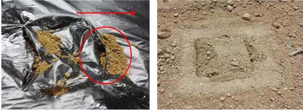
Fig. 140. State of plastic film and soil surface after verification test ( $V < R$ )
