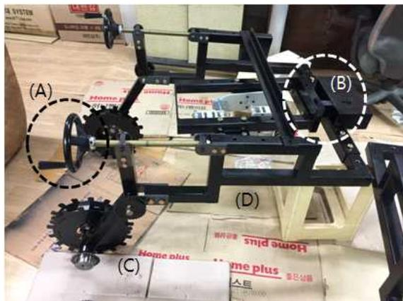
Fig. 213. Punching machine main frame of 3<sup>rd</sup> year automatic punching machine prototype, (A) height adjustment device, (B) width adjusting device, (C) driving wheel, and (D) punching machine main frame
