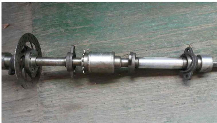
Fig. 211. Power transmission shaft of 3<sup>rd</sup> year automatic punching machine prototype
