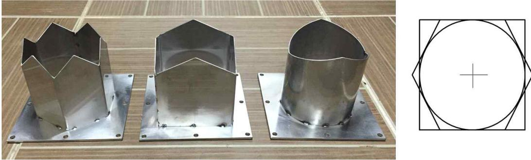
Fig. 143. Three different types of cutting knife and their edge angles of punching device (material ; STS-304)
