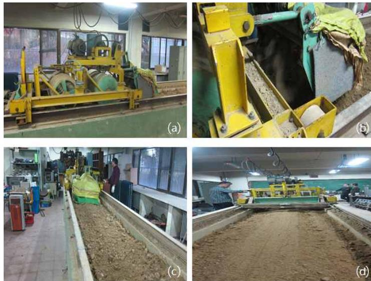
Fig. 113. Soil bin system, (a) View of soil process, (b) View of rotary tiller for soil preparation, (c) View of soil preparation, (d) View of soil after soil processing
