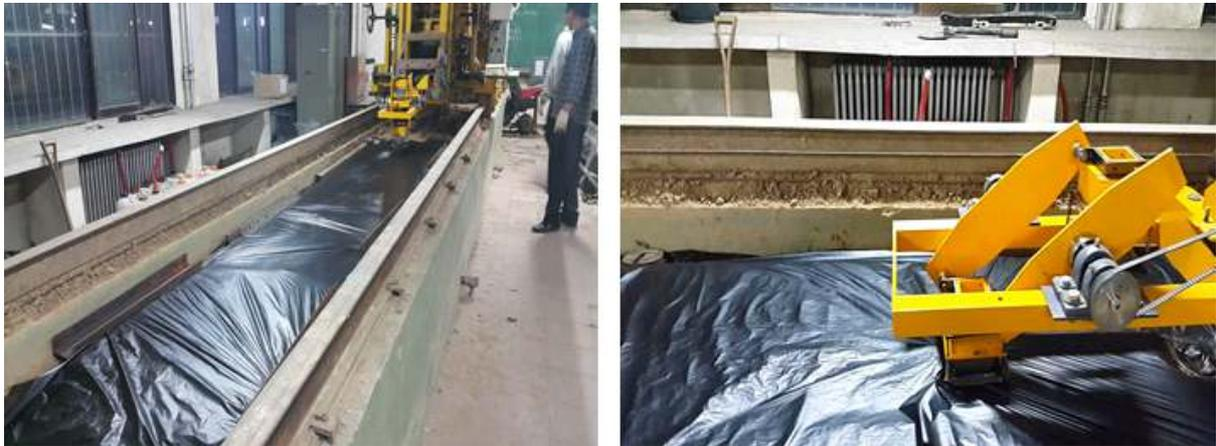
Fig. 115. Verification test of the circular-path type puncher
