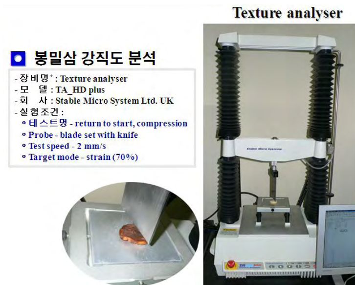
Fig. 3. Texture analyser for measuring the rigidity of fresh ginseng and honeyed ginseng.
