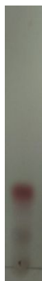
Figure 23. TLC analysis of compound K recovered by Prep TLC after enzymatic esterification with lipase (with a developing solvent of \text{CHCl}_3:\text{CH}_3\text{OH}:\text{H}_2\text{O} (13:2:0.3)).
