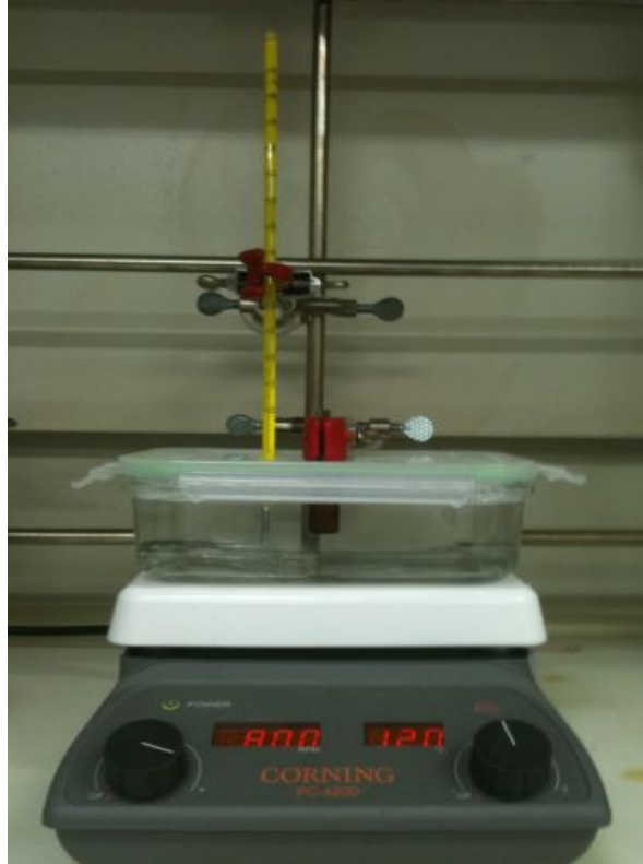
Figure 7. Stirred Enzyme reactor with immobilized lipase.
