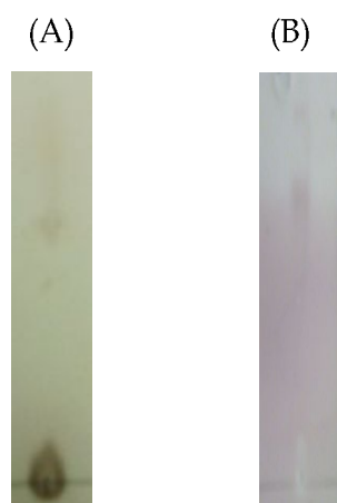
Figure 17. TLC analysis of esterification reactions of compound K (0.2%, w/v) with octanoic acid (6.4%, v/v) in isooctane:DMSO (31.25:1) at 96hrs using two different lipases (with a developing solvent of hexane:EA (30:1)); (A) Novozym 435, (B) Lipase GF.
