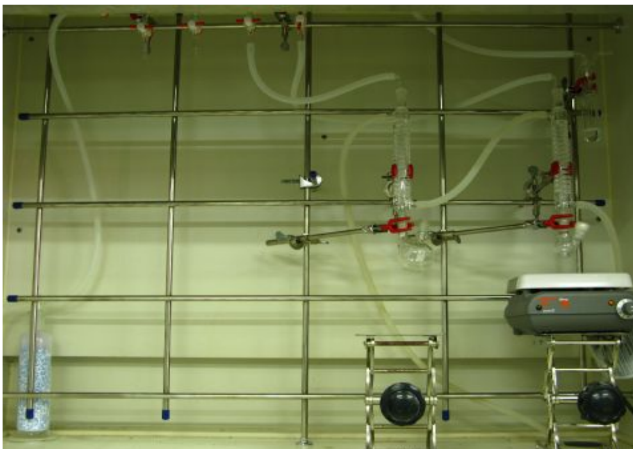
Figure 6. Chemical reactor for esterification reaction between compound K and oleic acid.
