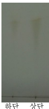
Figure 21. TLC analysis of fatty acyl compound K ester compounds separated by Prep TLC after solvent extraction (with a developing solvent of hexane:EA (30:1)).
