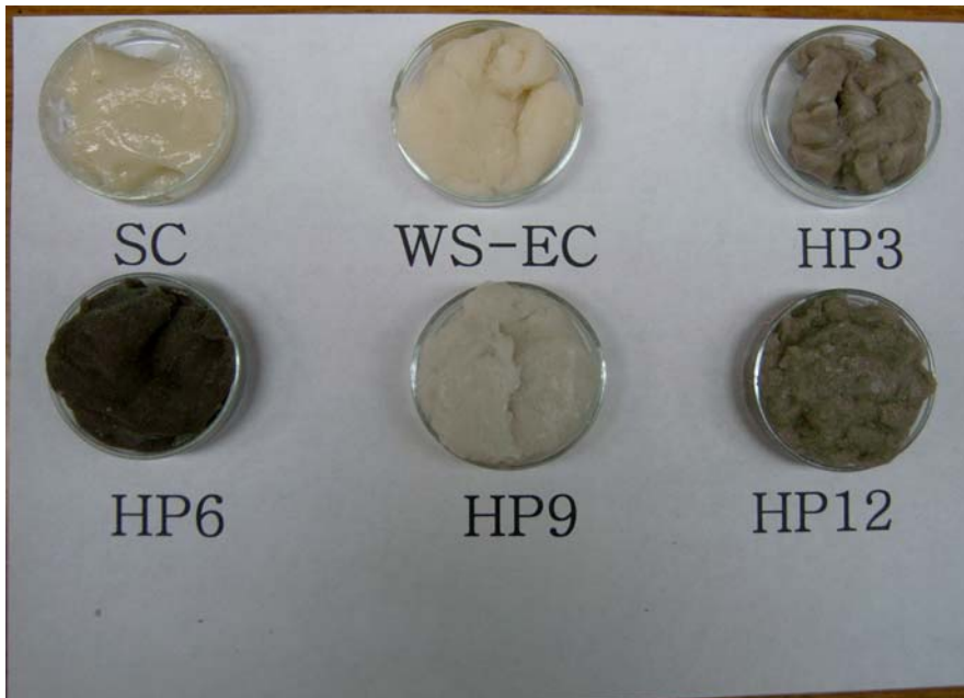
Fig. 33. Appearance of waxy starch dough after punching SC, control; WS-EC, raw waxy starch; HP3, 3% hydroxypropylated starch; HP6, 6% hydroxypropylated starch; HP9, 9% hydroxypropylated starch; HP12, 12% hydroxypropylated starch.
