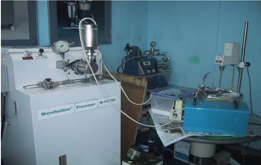
Fig. 20. High pressure microfluidization for the treatment of waxy rice starch.
