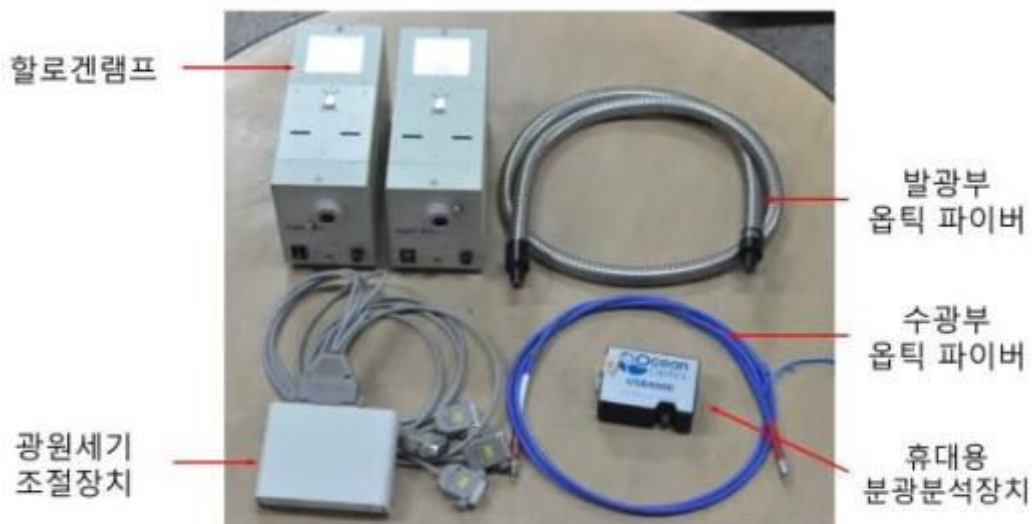
Fig. 58. Components of a prototype for nondestructive spectral measurements.
