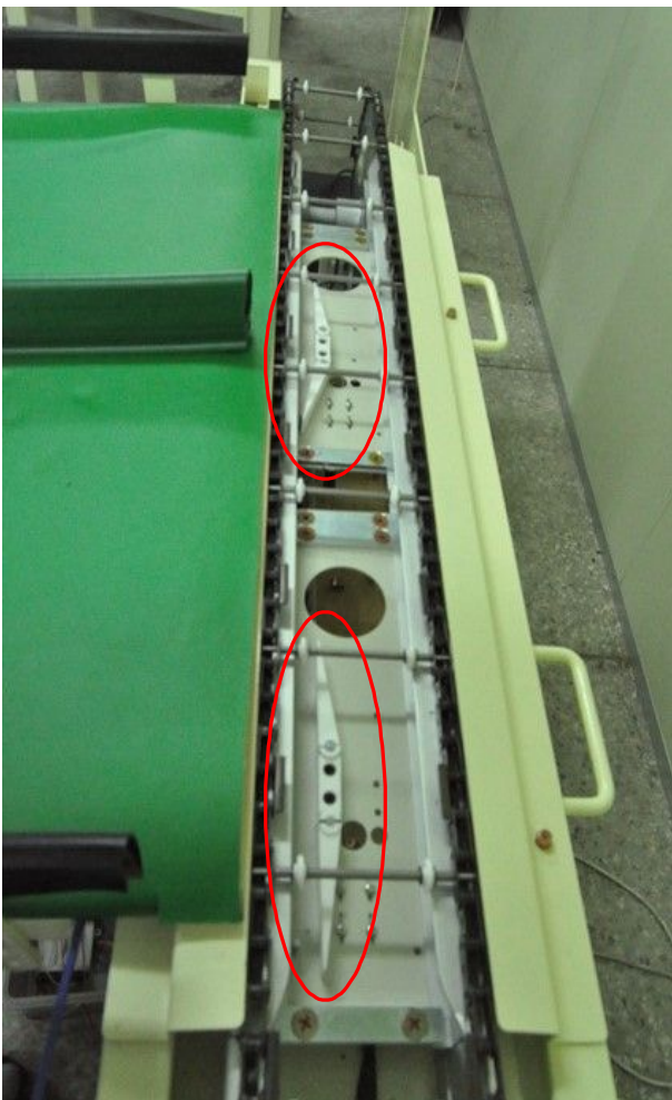
Fig. 62(b). Seed potato transfer container and solenoid valve of the developed sorting machine of seed potatoes.
