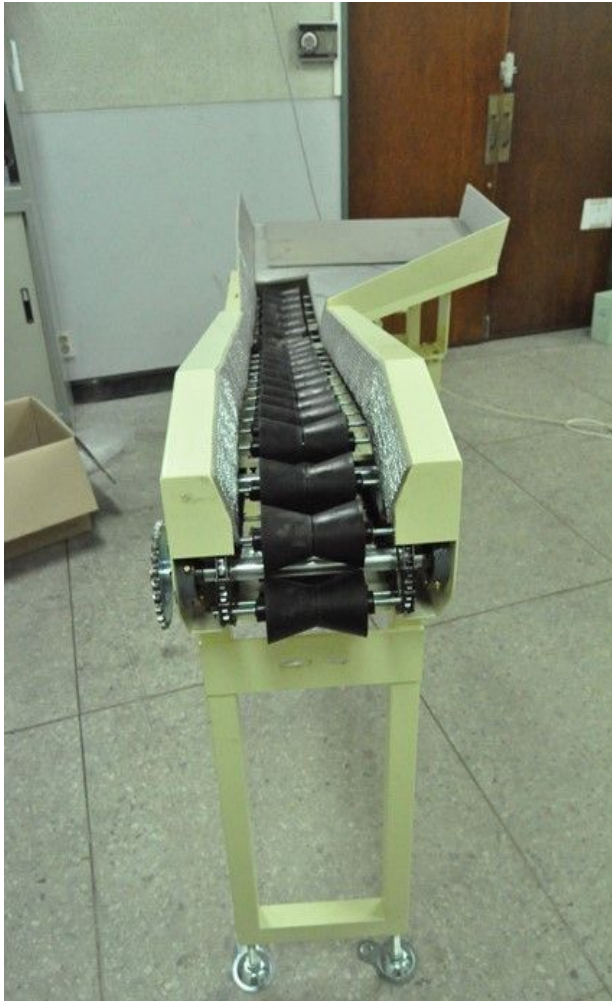
Fig. 62(a). Insert part of the developed sorting machine of seed potatoes.
