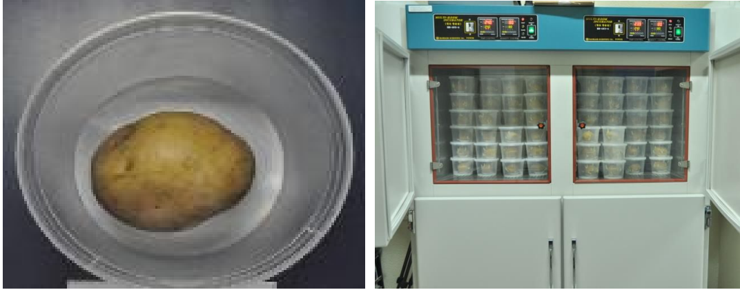
Fig. 11. Seed potato in plastic container and samples stored in a constant temperature and humidity chamber.
