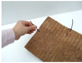
2. Fastening two sheets of coir tape.
