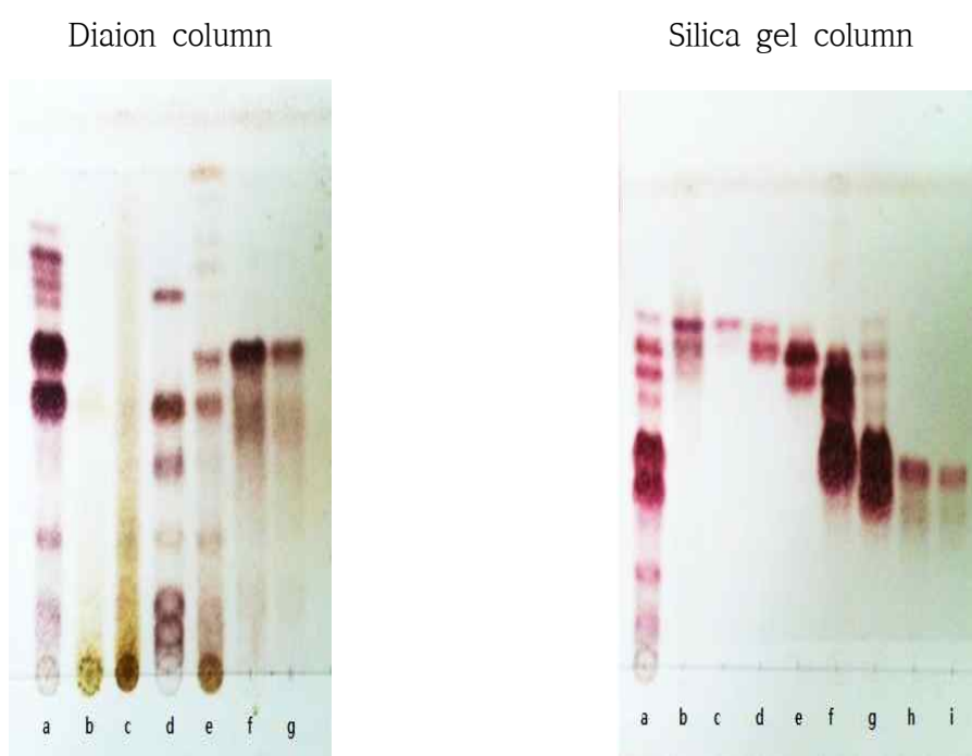
Fig. 1. TLC chromatogram of Black ginseng extract and compound I and ginsenoside Rg5, Rk1
