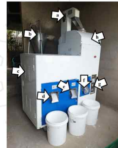
Figure 1. Parts of the LEE HWA LHP-200CM Corn Mill powered by 2.2 kW LEEHWA SE-2200 Electric Motor include the following: (a) Elevator assembly, (b) Cyclone separator, (c) Degreaser and screen chamber, (d) Grit #10-12 outlet, (e) Grit #14-18 outlet, (f) Corn flour outlet, (g) On/off switch, and (h) Milling chamber.
