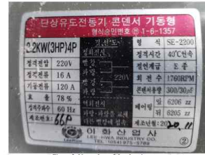
Figure 3. Nameplate of the electric motor.
