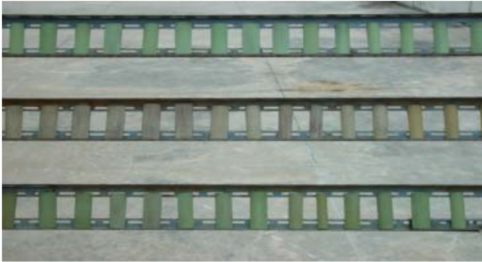
Figure 4-1. View of the preservative-treated bamboo samples exposed to the weather.
