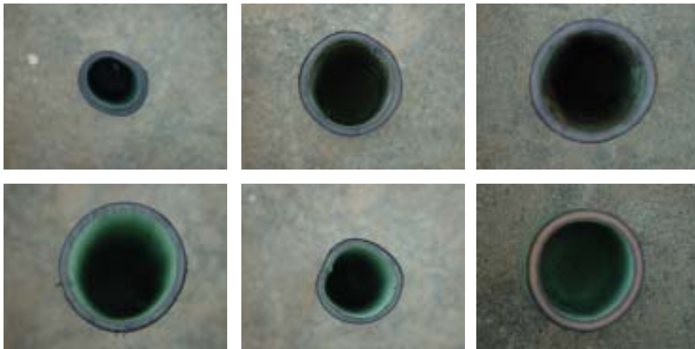
Figure 3-24. Photographs showing CCA penetration of dip-treated bamboo samples (lower) and dip-treated bamboo samples after pressure treatment - Left: Giant timber bamboo, Middle: Hachiku bamboo, and Right: Moso bamboo.
