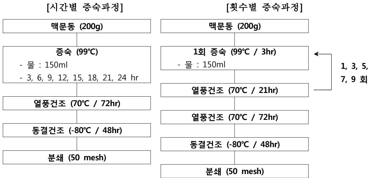
Fig. 1. Schematic diagram of steaming and drying process of Liriopsis tuber
