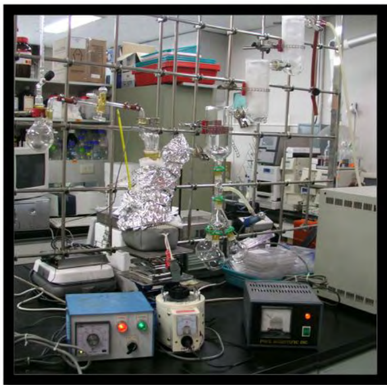
Figure 34. Distillation system for separation of policosanol-DHA ester from reaction mixture
