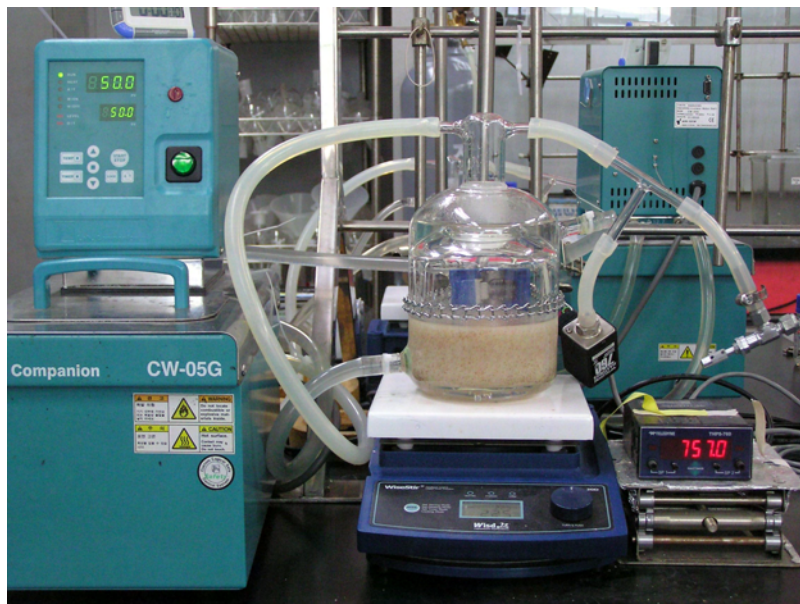
Figure 20. Bulk scale reaction system for synthesis of policosanol-DHA ester by lipase-catalyzed esterification
