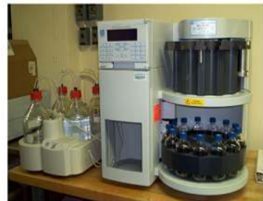
Accelerated solvent extraction module (Dionex Model 300) used for the SWE of fruit berry substrates.
