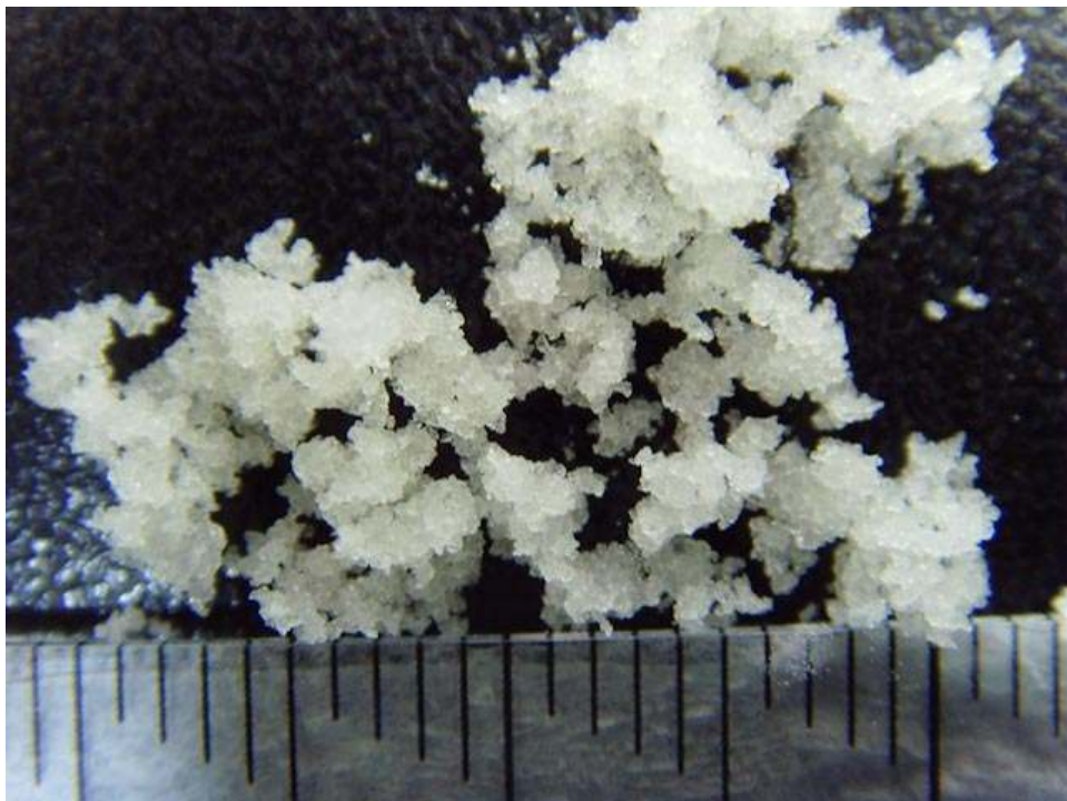
그림 45 Immobilized PLA2 using Crosslinked enzyme matrix bound to silica method
