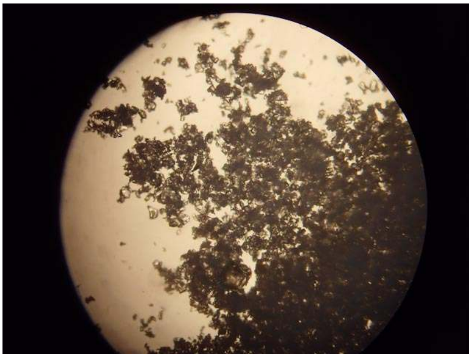
그림 47 Optical microscopic image of immobilized PLD using Crosslinked enzyme matrix bound to silica method (magnification : x160)
