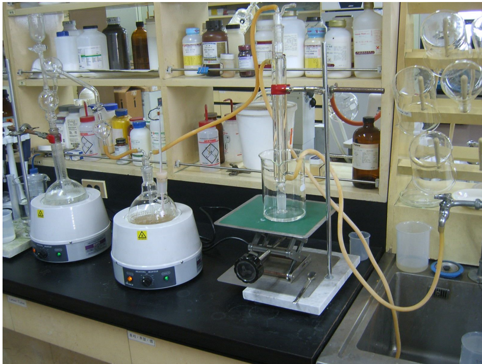
Figure 9. Equipment for sublimation of HCN.
