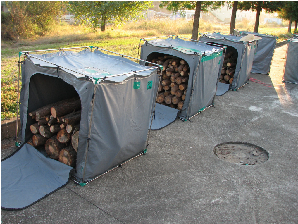
Figure 6. Tapaulin fumigation chamber (1 m 3 ).
