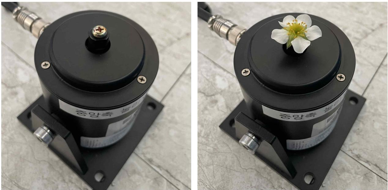
**Fig. 8.** Vibration generator (A) and strawberry flower attached to the generator (B).
