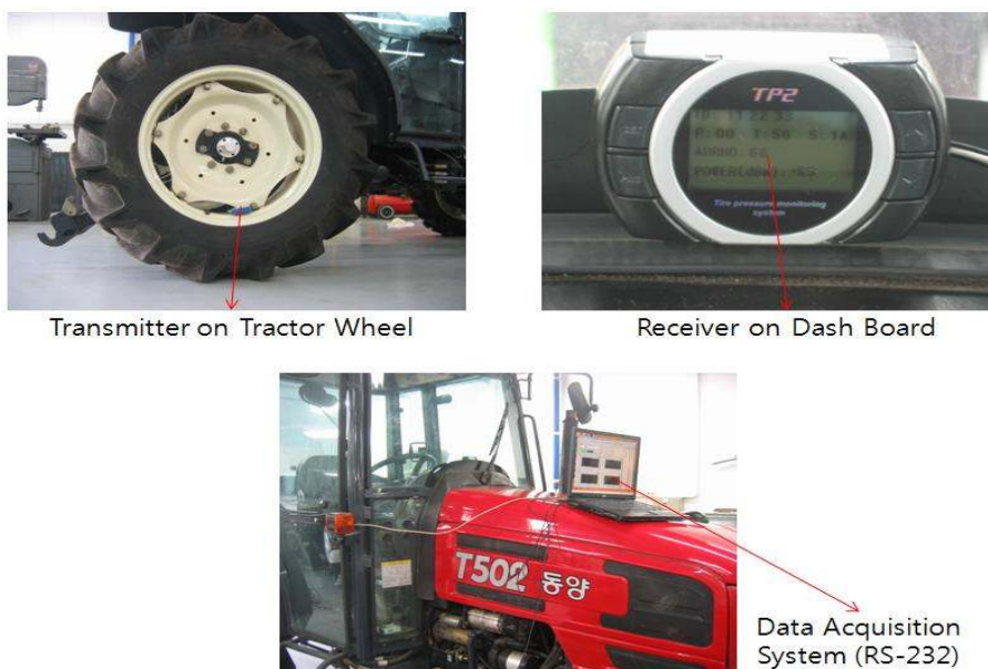
Fig. 3.22 RSSI measurement setup in tractor. (stationary)
