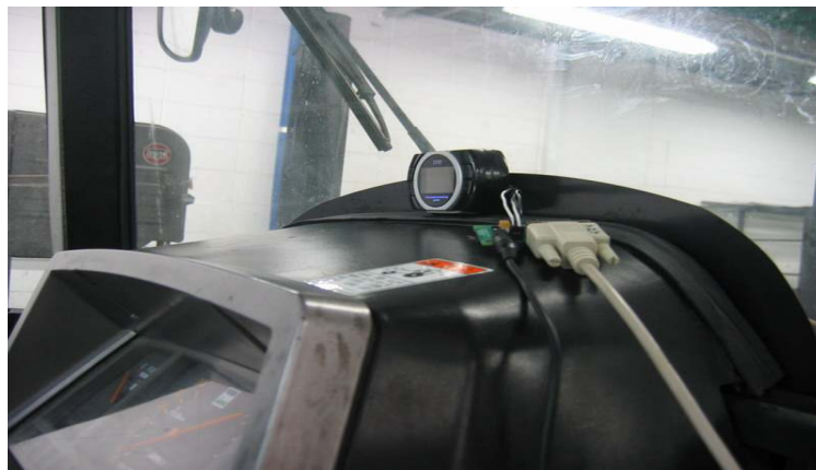
Fig. 5.6 Controller installed on the instrument panel of T502 tractor.
