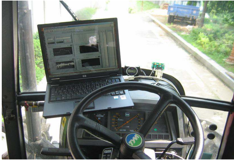
Fig. 3.23 RSSI measurement setup in tractor. (driving)
