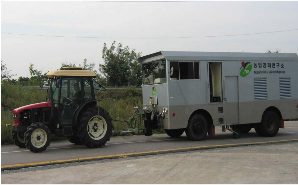
Fig. 5.13 Drawbar performance test by a dynamometer car on test track.
