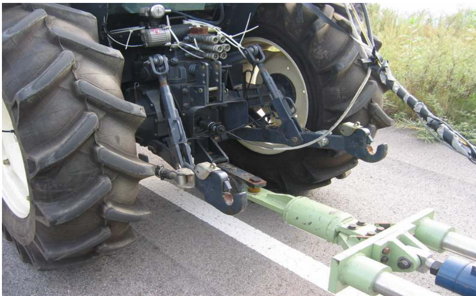
Fig. 5.14 Drawbar connected to dynamometer car.
