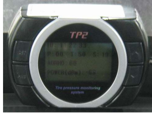
Fig. 5.3 Control and display unit.
