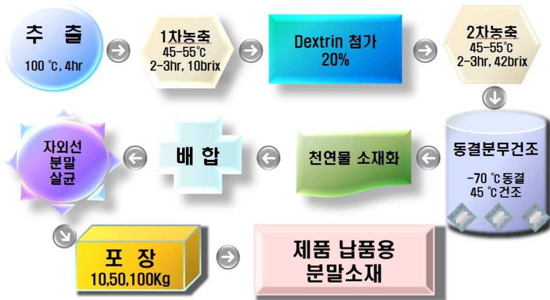
Fig. 2-5. The scheme for manufacture of Wa-song naturally.
