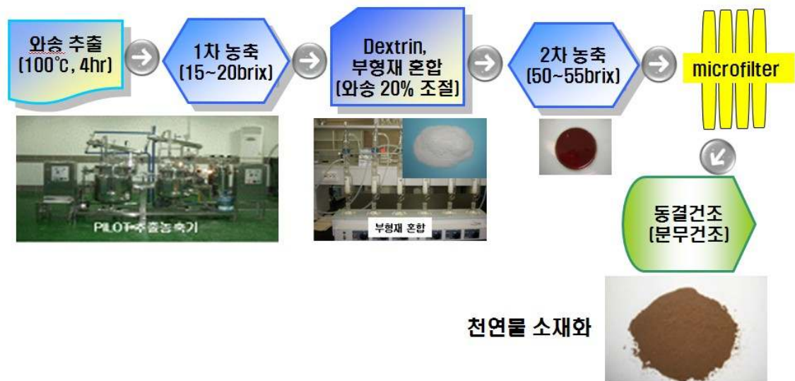
Photo. 2-6. The plan for manufacture of Wa-song naturally.
