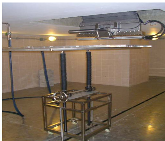
Fig. 4.29. Cart system of electron accelerator(2.5 MeV).
