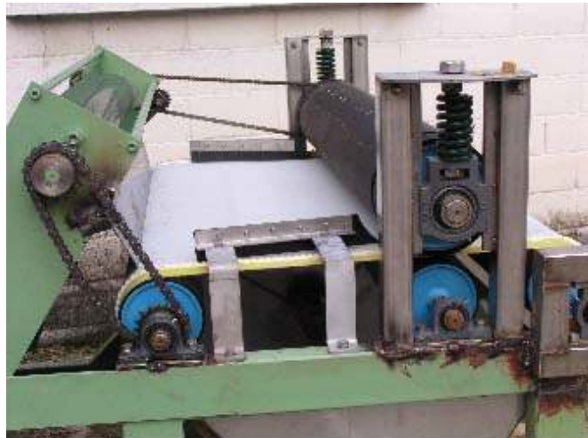
Fig. 3-11. Picture of the compress type roller dehydrator of the 2nd prototype fecal-sawdust based dehydration and sterilization system.
