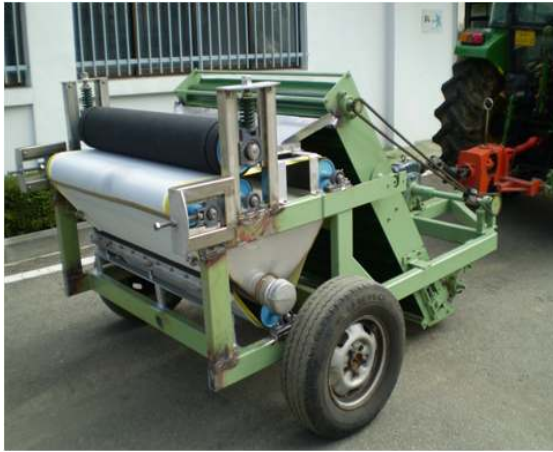
Fig. 3-9. Picture of the 2nd prototype fecal-sawdust based dehydration and sterilization system for preventing mastitis in dairy cows.
