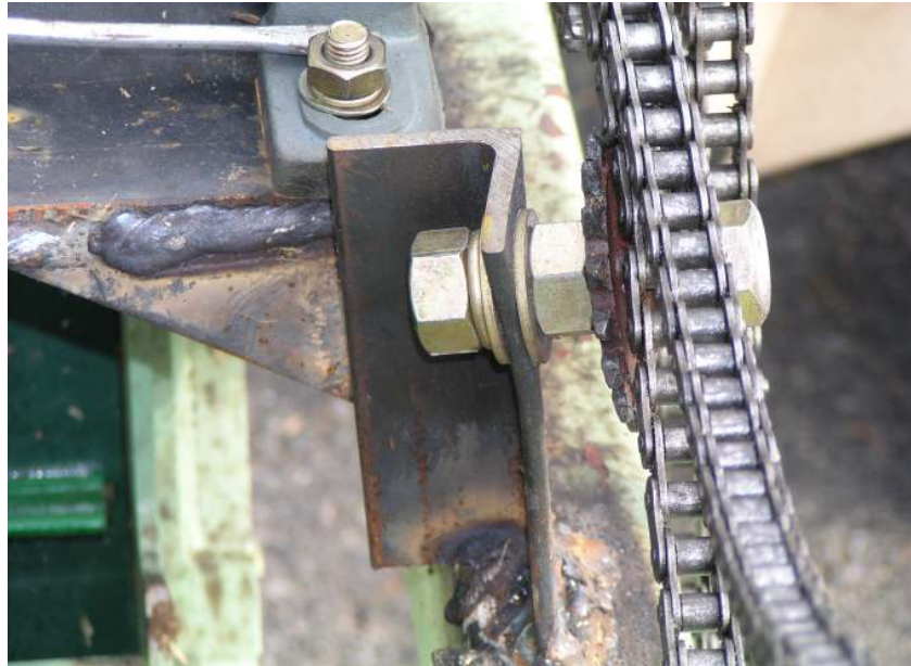
Fig. 3-25. Picture of a damaged sprocket.
