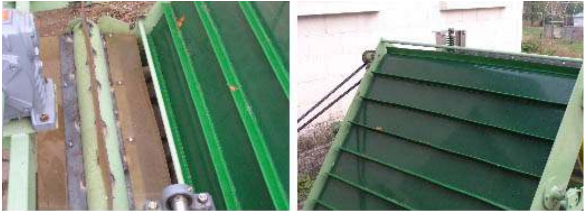
Fig. 3-10. Inlet of the 2nd prototype fecal-sawdust based dehydration and sterilization system (left) and conveyor belt (right).
