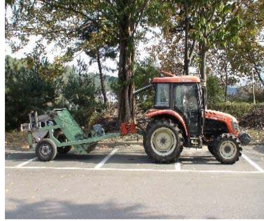
Fig. 3-9. Picture of the 2nd prototype fecal-sawdust based dehydration and sterilization system for preventing mastitis in dairy cows.
