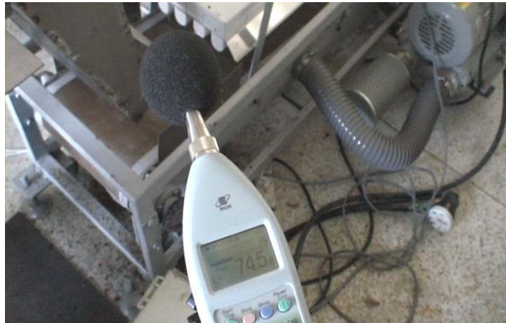
Fig. 3-4. A picture of noise measurement of the preliminary sterilizer.
