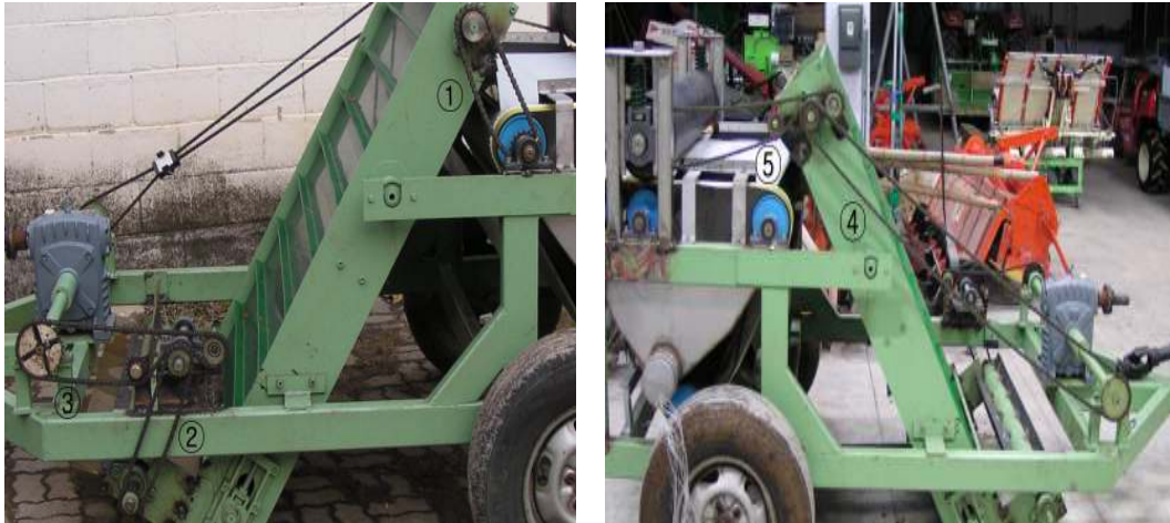
Fig. 3-24. The picture of the 1st prototype fecal-sawdust based dehydration and sterilization system for preventing mastitis in dairy cows.
