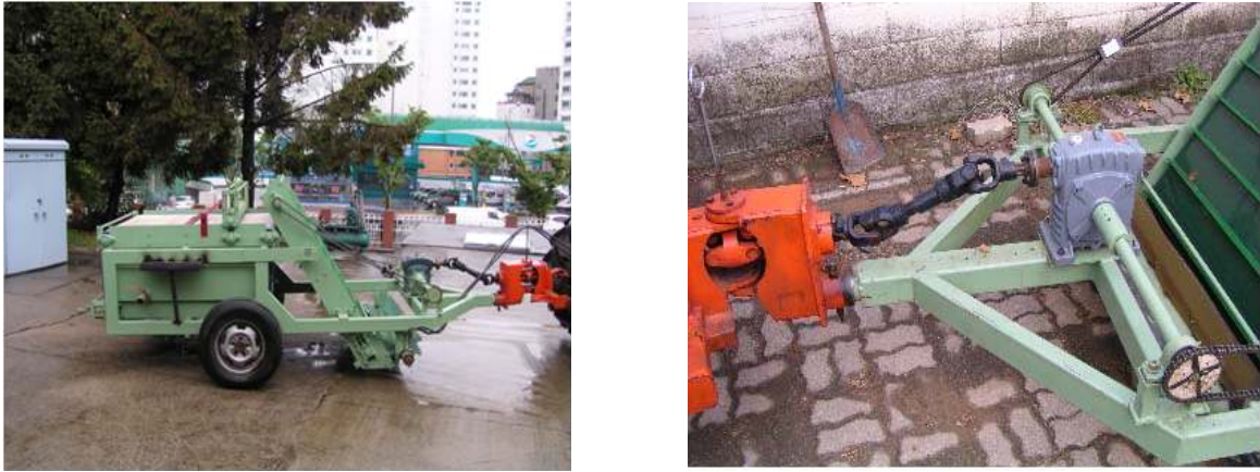
Fig. 3-8. Pictures of the 1st prototype fecal-sawdust based dehydration and sterilization system for preventing mastitis in dairy cows (left) and its power transmission (right).
