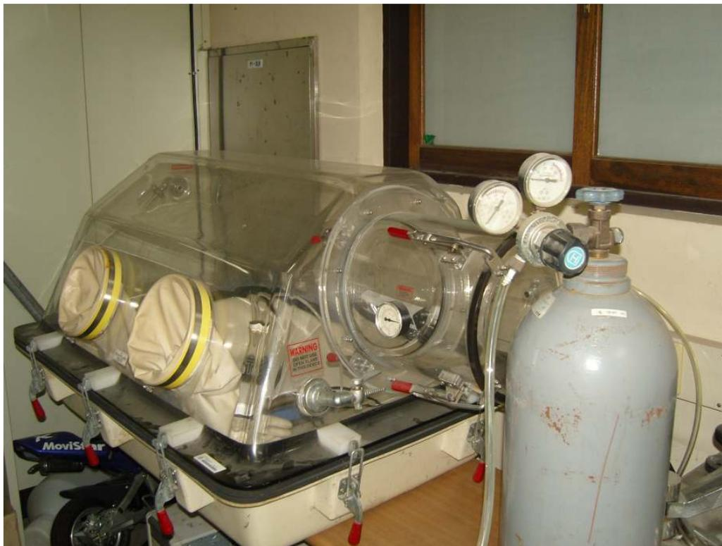
Figure 2-2. Picture of anaerobic chamber used in this study to deliver inoculum of MCR to BMP test flask
