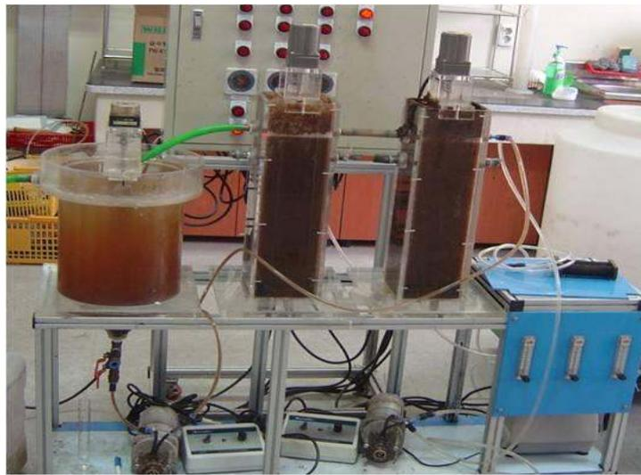
Figure 4-1. 2-stage intermittently aerated activated sludge system
