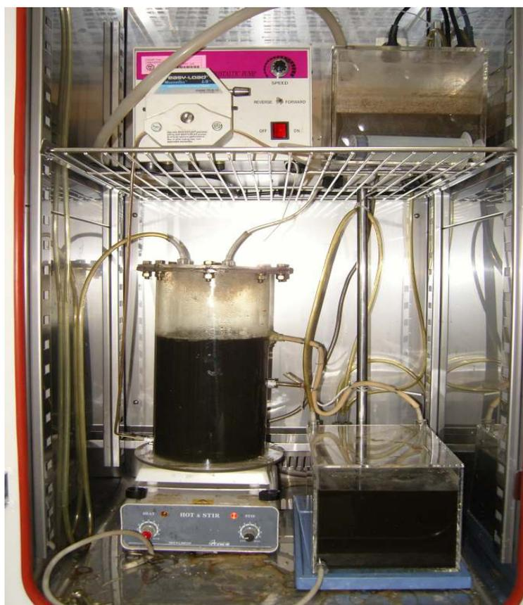
Figure 3-1. Configuration of completely stirred tank reactor for thermophilic anaerobic bioreactor for treating swine and mixture wastewaters (swine wastewater : leachate from sood waste : sewage sludge = 1 : 1 : 1)
