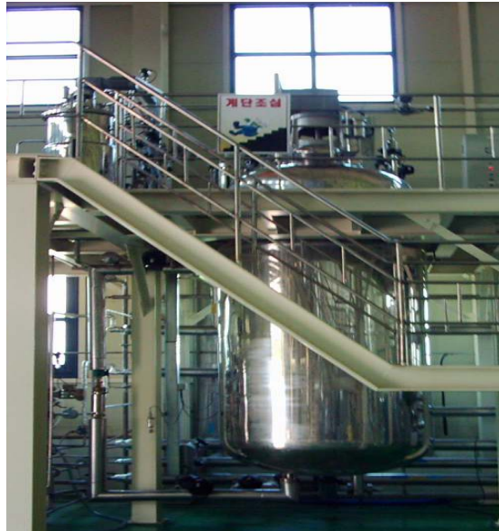
Figure 4. Feature of fermenter (5 kl) for the production of submerged-liquid culture of Agaricus blazei .
