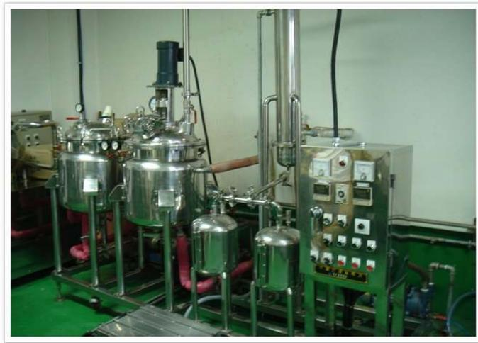
Fig. 6. Vacuum evaporation of starch syrup made from *Ogaza* extract
