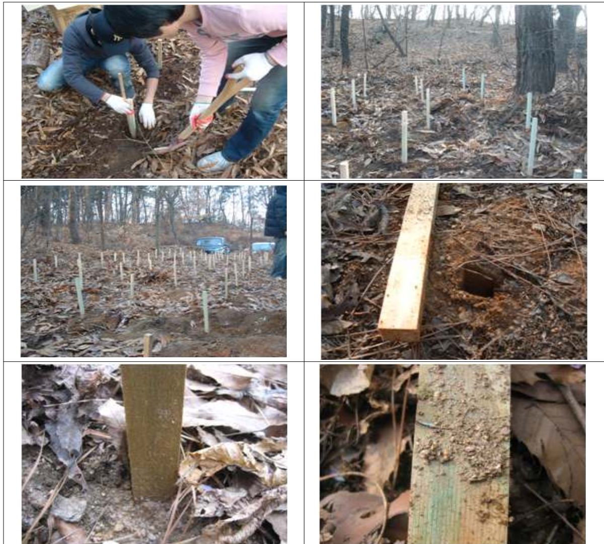
Figure 53. Images of the field test for the fence poles treated with okara-based wood preservatives in Chungbuk National University (Cheongju, Chungbuk, Korea).
