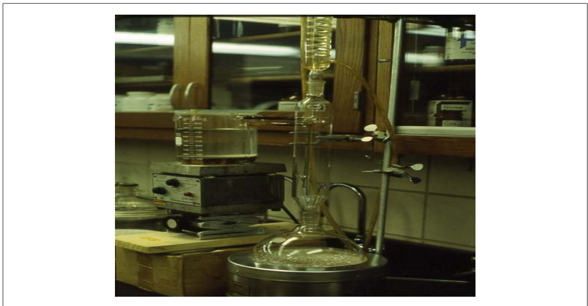
Figure 29. The image (left) and schematics (right) of the extraction apparatus for studying leachability of wood preservatives.
