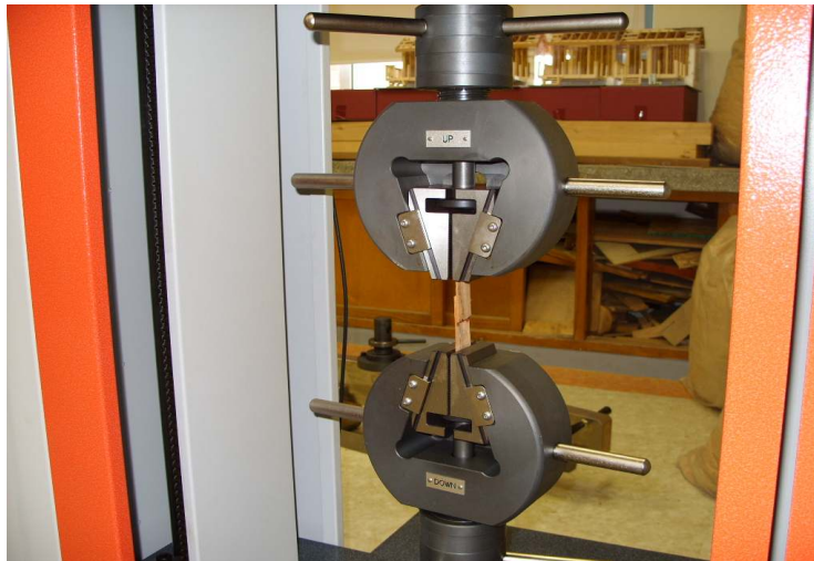
Figure 23. Test configuration for measuring lap joint shear tensile strength.
