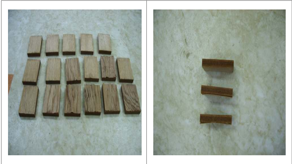
Figure 20. Images of specimens prepared for the determination of wet wood failure – excellent (top), good/fair (middle) and poor (bottom).
