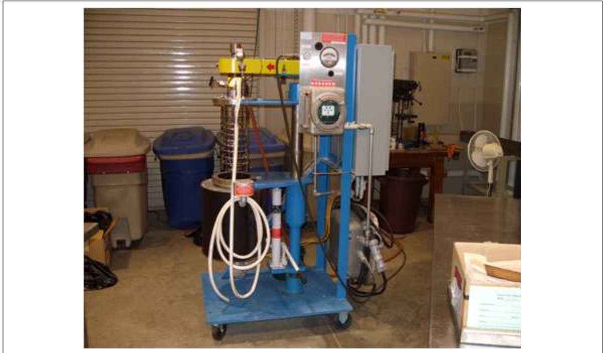
Figure 51. Pilot-scale reactor for the preparation of okara hydrolyzates in Iowa State University (Ames, Iowa, U.S.A.).
