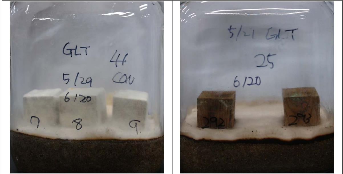
Figure 35. Features of Control (left) and wood blocks treated with \text{CuSO}_4 \cdot 5\text{H}_2\text{O} /Okara hydrolyzates (right). The wood blocks treated with CS/OK were subjected to leach at 70°C water for 72 hours. Both types of wood blocks were exposed with the brown-rot fungus Gloeophyllum trabeum for 12 weeks.
