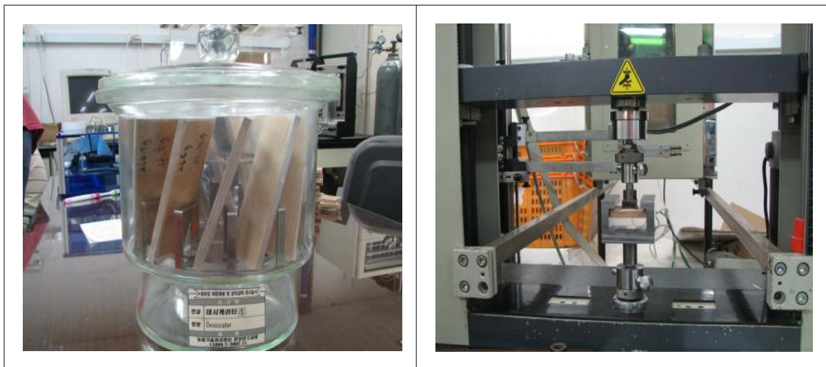
Figure 17. Desiccator method and glueline bonding strength configuration.
