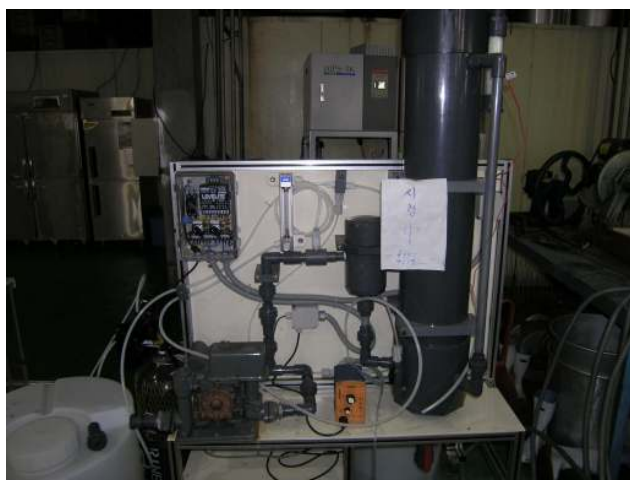
Fig. 2. Aqueous \text{ClO}_2 generator used in this experiment
