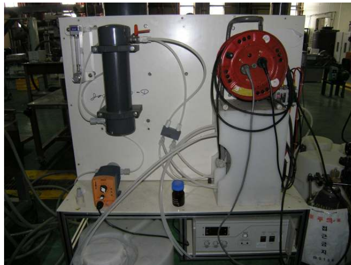
Fig. 4. Electrolyzed-water generator used in this experiment.
