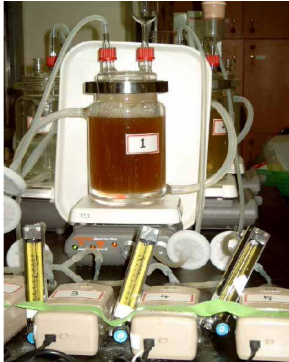
Fig. 4. Fermenter for manufacturing vinegar
