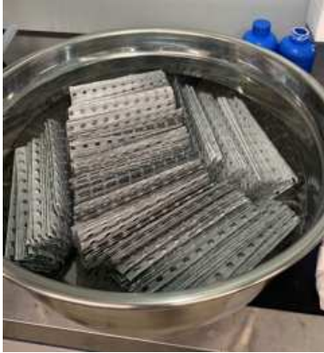
(a) 농도 2% PHPS 용액 Dip coating
