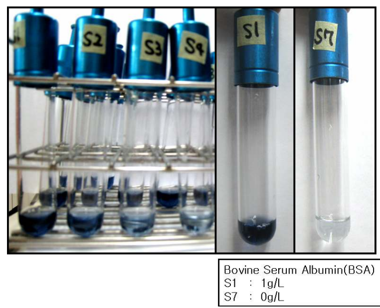
Figure 2-58. Protein determination contained in the fermentation broth by use of Lowry method (Bovine serum albumin was used as a standard for the determination of protein amounts)
