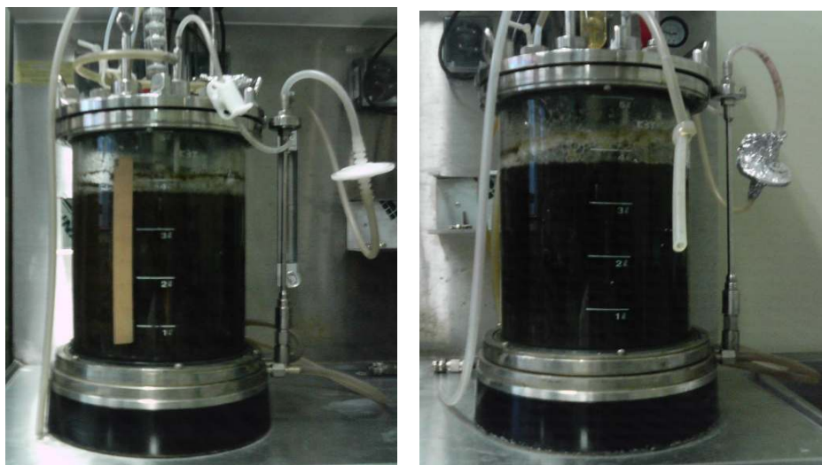
Figure 8. The submerged liquid culture in the 5 L fermenter. Left; 0.25% (w/v) green tea included, Right; 0.5% (w/v) green tea included.
