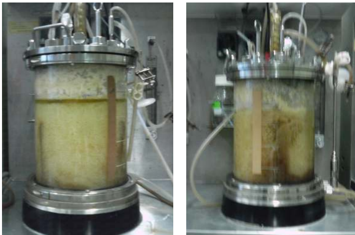
Figure 9. The submerged liquid culture in the 5 L fermenter. Left; 0.5% (w/v) onion included, Right; 1.% (w/v) onion included.
