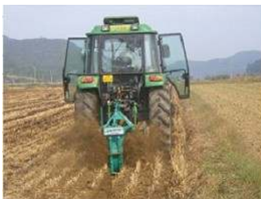
Fig. 5-7 A covering device, soil covering and draining ditch work in paddy field.
