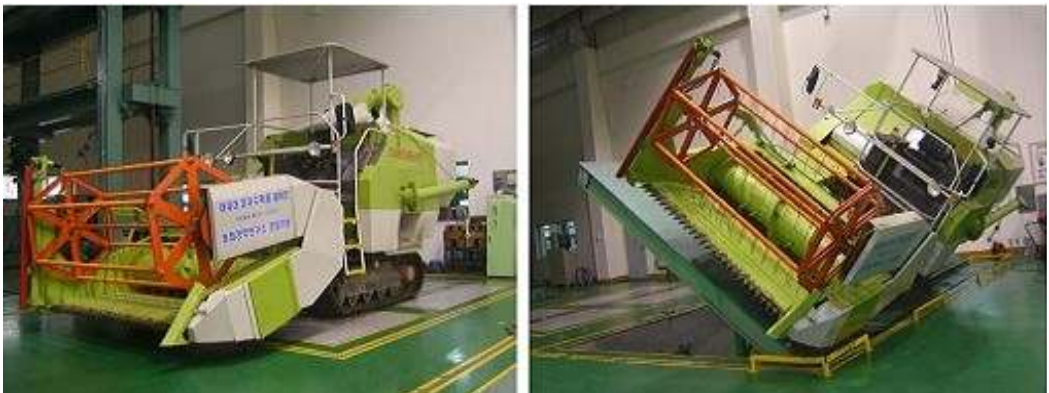
Fig. 5-38 Measurement of weight and static turn-over angle.
