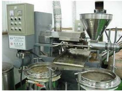
Figure 3. Expeller type Oil Expressions-DONG KWANG OIL MACHINE.
