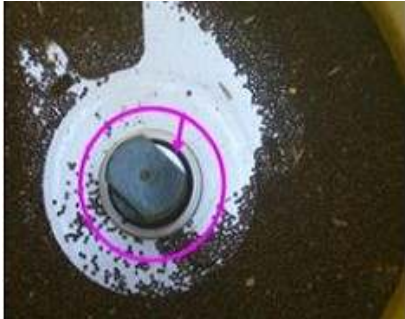
Fig. 5-22 Chink in the shaft of agitator. Fig. 5-23 View of damaged rapeseed.
