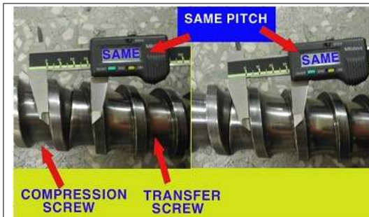
Figure 6. inside Expeller - screw.
